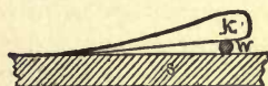
FIG. 15.—Diagram illustrating the position of the knife in sharpening. k , knife; s , oilstone; w , wire.
