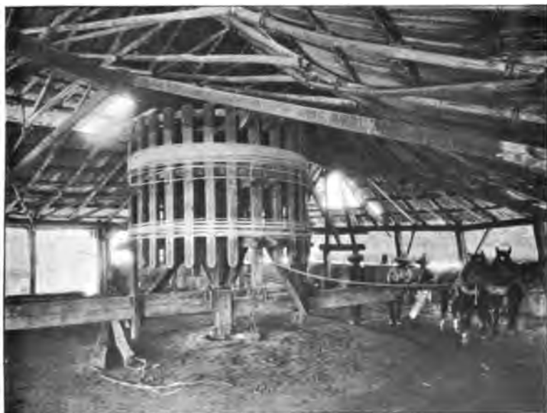
PRIMITIVE FORMS OF MINING.—Raising ore from the shaft by horse-whim.
