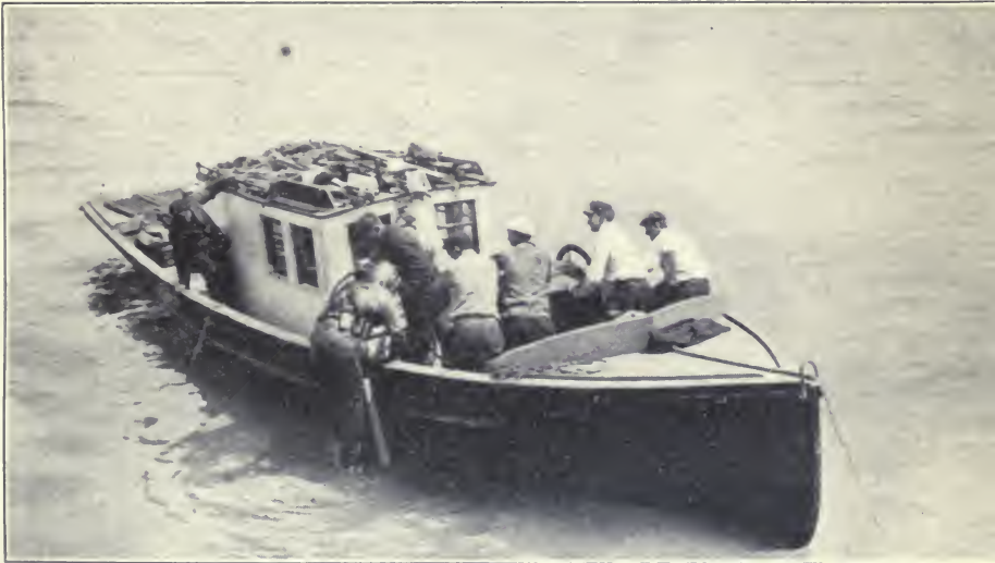
Diver descending from a United States Survey power boat to ascertain the nature and conformation of an obstruction to navigation located by a drag.
