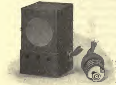
FIG. 65.—Incandescent Electric Lamp for Use with Microscope.
