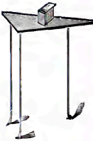
FIG. 26.—Imbedding-Table. Tines should be two rectangular bones (about 3/32 x 1/8 cm.) to contain paraffin. When in use the bones are so placed on the imbedding-table that the paraffin in one end remains melted; in the other, solid. Regulate the temperature by placing the flame at the proper distance under the acute angle of the table. It is best, when gas is used, always to turn on the gas completely and then regulate the height of the flame by means of a clamp on the rubber tubing which conducts gas to the burner.
