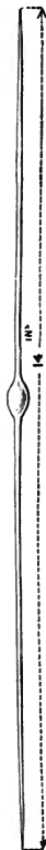
FIG. 5—A CAPILLARY PIPETTE, DRAWN OUT INTO FINE POINTS; LENGTH ABOUT 12 TO 14 INCHES.
