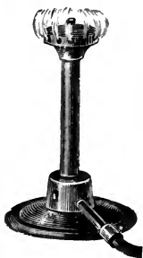
FIG. 2.—A BUNSEN BURNER WITH ROSE FOR BOILING FLUIDS IN TEST-TUBES.
