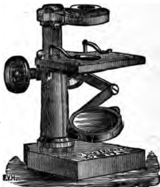
FIG. 8a. — Simple Microscope with Special Mechanical Mounting to Hold and Focus the Magnifier and to Support and Light the Object.
