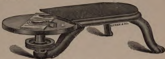
Fig. 38a. Turn-Table for Sealing Cover-Glasses and Making Shallow Mounting Cells. (Queen & Co.)
