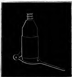
Achromatic Condenser, consisting of a French combination mounted in a simple tube and focussed with a lever motion, as suggested by Professor Quekett.
