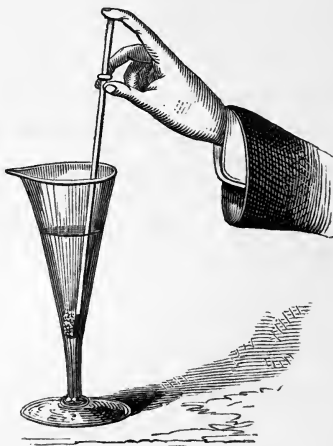
Conical Glass, for allowing deposits from fluids to subside. The drawing shows the manner in which a portion of the deposit is to be removed with the pipette.
