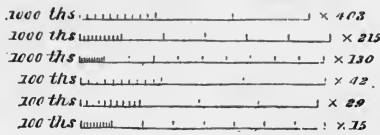
1000ths and 100ths of an English inch magnified in various degrees. The smallest divisions indicate 10,000ths and 1000ths of an inch.
