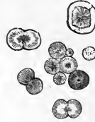
Crystals of carbonate of lime in Canada balsam, seen by transmitted light, \times 215 .
