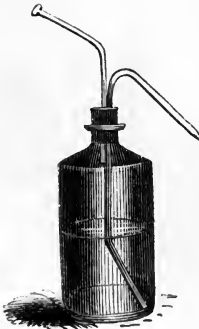
Wash - bottle for washing preparations, a stream of water is projected from the orifice of the pipe, when air is blown into the upper tube.
