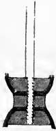
Section of piston of injecting syringe, showing the manner in which the leather is applied.
