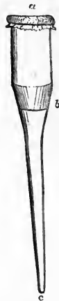
Pipette serving as the stopper to the bottle. a. Vulcanized India - rubber, by pressing which, fluid may be expelled from the tube. b. Ground to fit the neck of the bottle. c. Orifice.
