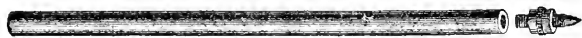
FIG. 136. Writing diamond for writing numbers and labels on glass slides, cutting cover-glasses, etc. (Queen & Co.).
