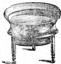
FIG. 154. Tripod magnifier. This serves fairly well as a focusing glass, but is inferior to the one shown in Fig. 153.
