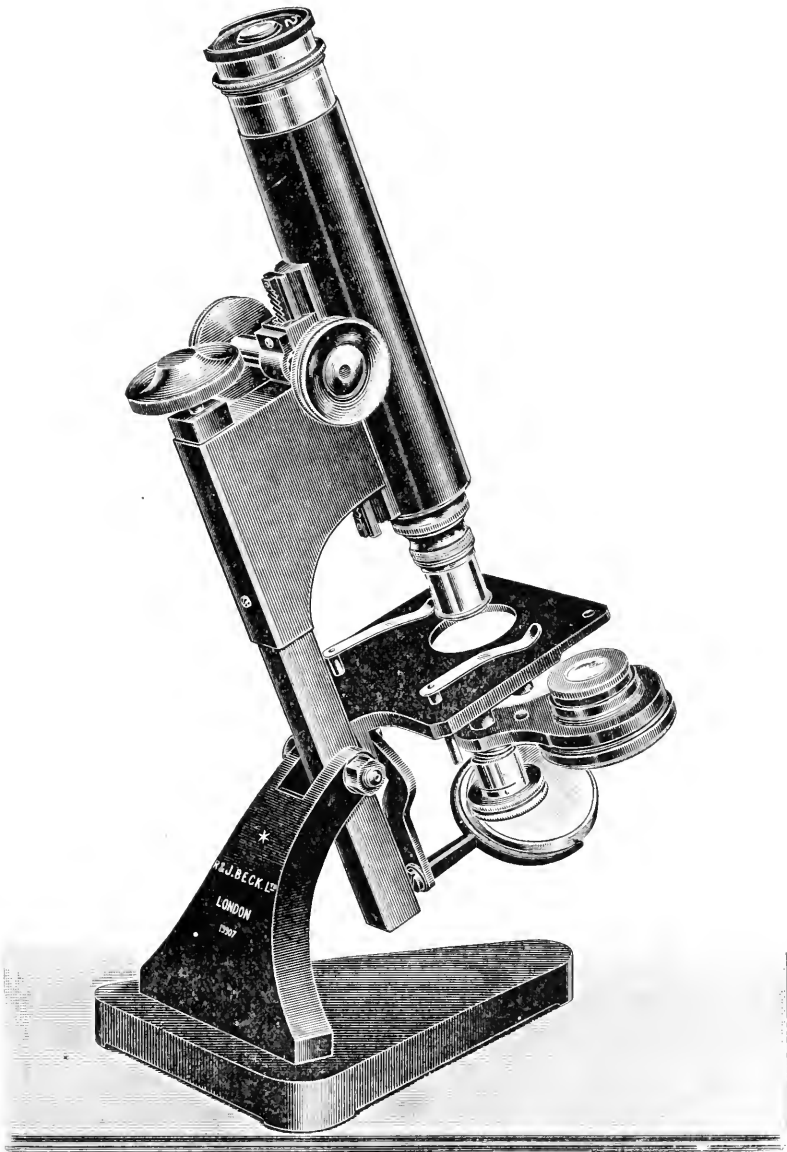
FIG. 79. Beck's Star Microscope.
