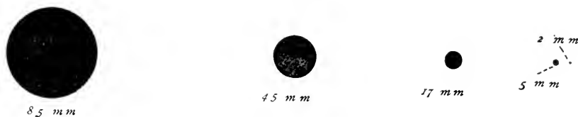
FIG. 37. Figures showing approximately the actual size of the field with objectives of 85 mm., 45 mm., 17 mm., 5 mm., and 2 mm., equivalent focus, and ocular of 37\frac{1}{2} mm., equivalent focus in each case. This figure shows graphically what is also very clearly indicated in the table (§ 17).
