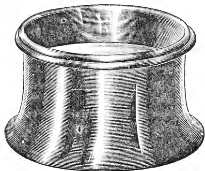
FIG. 155. Engraving glass to serve as a bull's eye condenser. (From the Bausch and Lomb Optical Co.)
