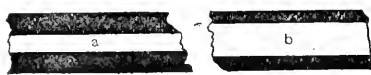
FIG. 89. Solid glass rod showing the appearance when viewed with transmitted, central light, and with an objective of medium aperture.
