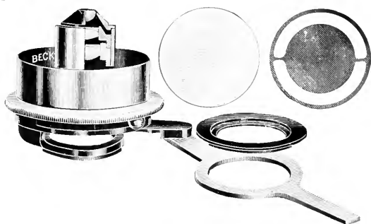
FIG. 247.—Beck's condenser with N.A. 1\cdot0 .
