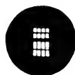
FIG. 355.—Image at the back of the objective when daylight and a plane mirror are used.
