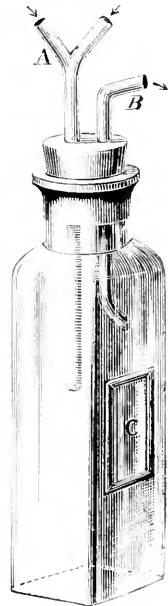
FIG. 409.—Arrangement for the orientation of objects in paraffin.
