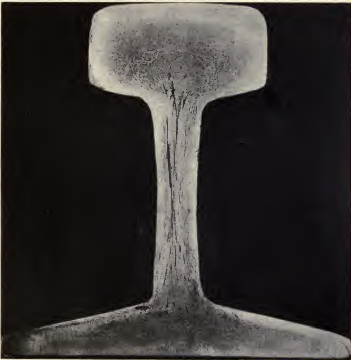
PHOTOGRAPH NO. 20. Cross section of steel rail showing segregation in center of head, web, and base.
