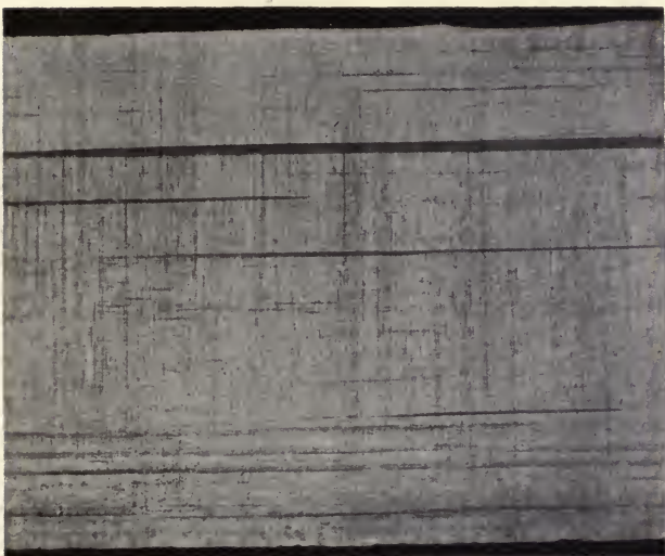
PHOTOGRAPH NO. 25. Dark streaks in steel rail.
