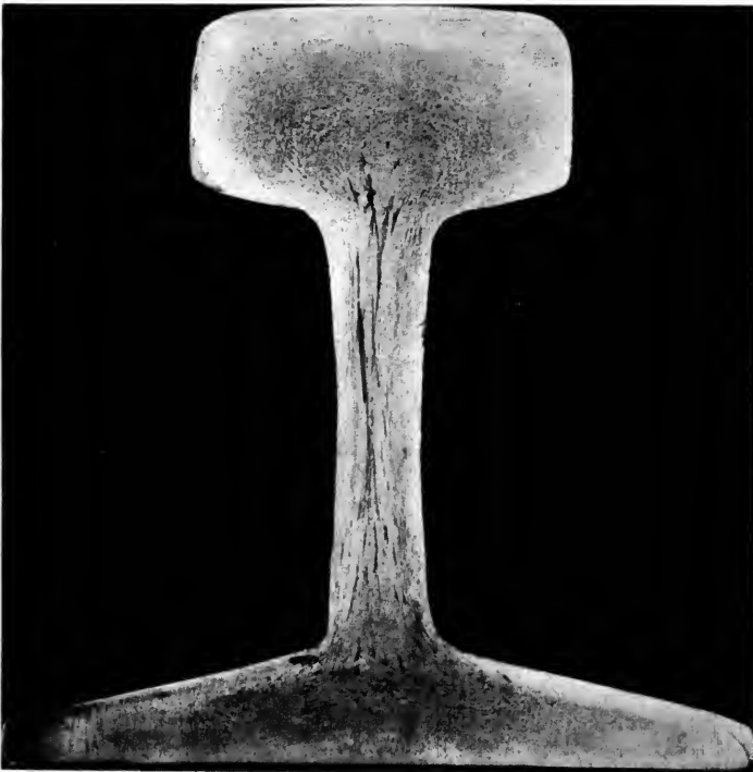
PHOTOGRAPH NO. 20. Cross section of steel rail showing segregation in center of head, web, and base.
