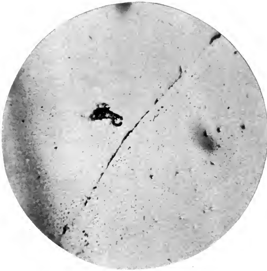
PHOTOGRAPH NO. 42. X50. Slag in 10-inch rifle, unetched.
