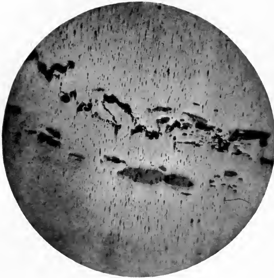
PHOTOGRAPH NO. 54. X50. Twelve-inch gun. Slag in unetched specimen.
