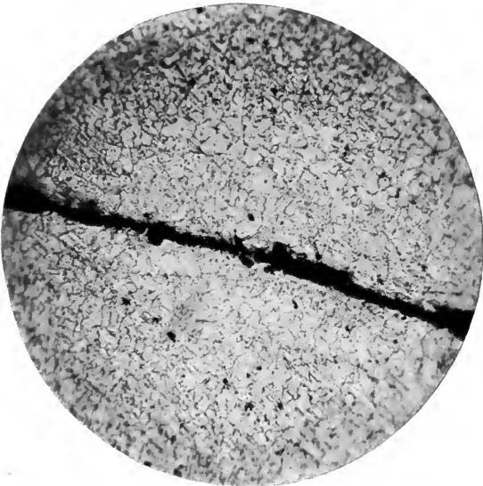
PHOTOGRAPH NO. 43. X50. Slag and decarbonized area in 10-inch rifle.
