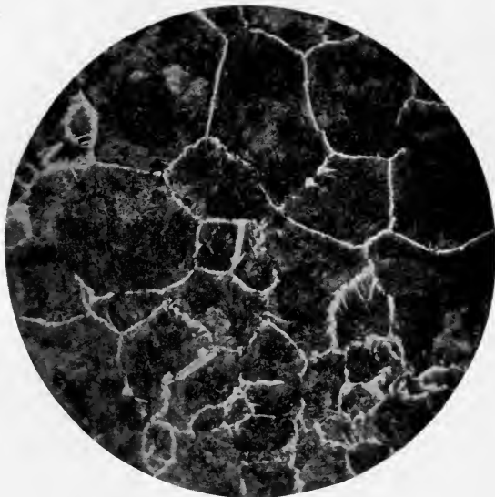
PHOTOGRAPH NO. 30. X75. Coarse microstructure in gun steel.
