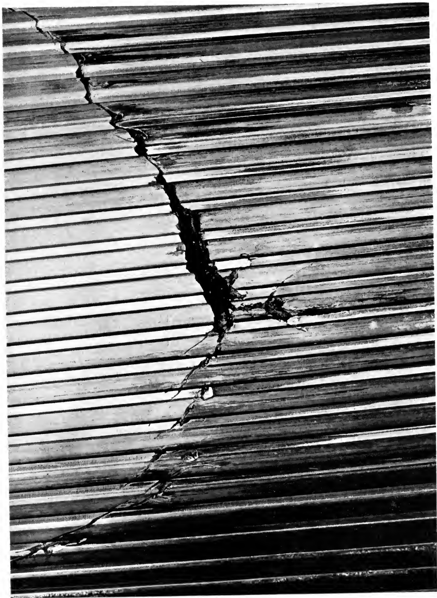
PHOTOGRAPH NO. 37. Crack in 10-inch rifle.
