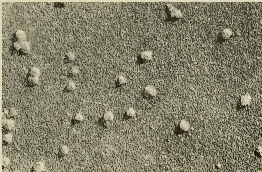
Fig. 3. An electron micrograph of a central portion of a sprayed droplet showing RNP particles magnified 170,000 times. The smallest particles are about 200 Å in diameter, the largest about 250 Å. From the shapes of their shadows it is estimated that their thicknesses are about 75 per cent as great as their diameters. Taken on a Siemens Elmiskop I by Professor Paul Kaesberg.
