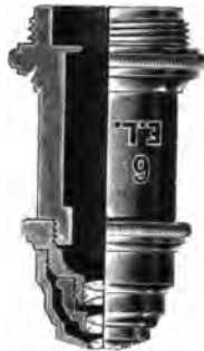
Fig. 815. Leitz'sches Achromat 6 f = 4,0 mm U = 0,82 "
