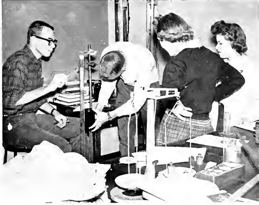
Students in physics class use a resonance apparatus to measure the velocity of sound in air.
