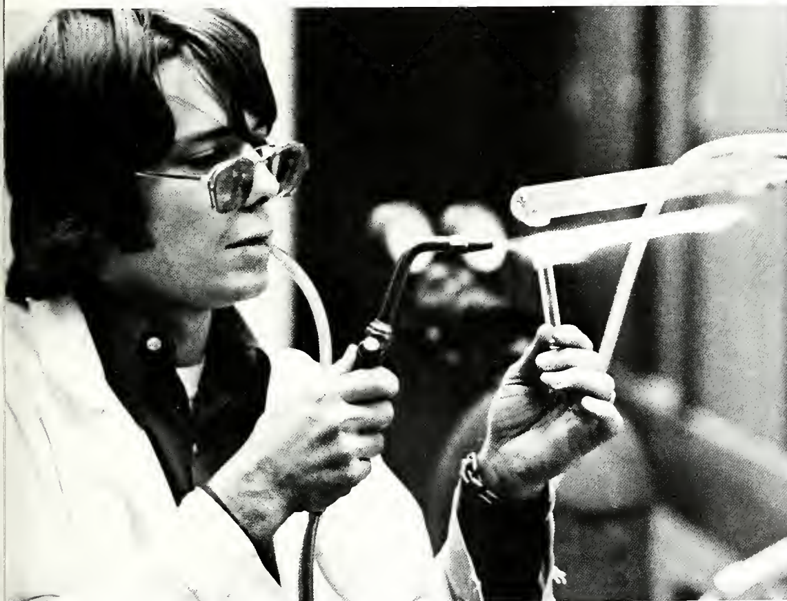
Dr. Tom Badgett, assistant professor of chemistry, demonstrates the technique used in forming glass tubings.
