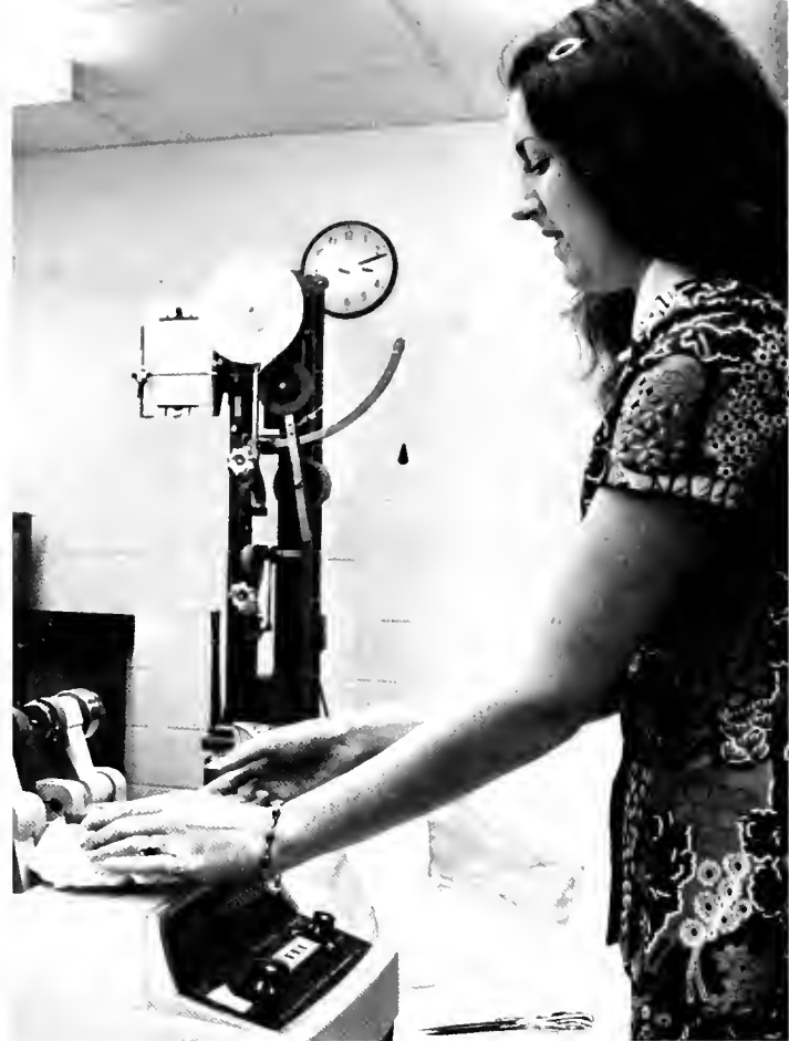
Pam Caldwell tests the abrasion resistance of cloth with the use of the Taber Abraser.
