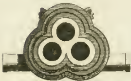
Section of the breech of the Triple Cannon.
