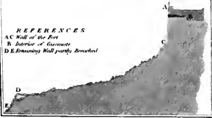
Section thro' the Breach & Casemates on the E. Side of the FORT.
