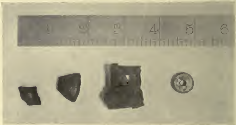
FIG. 7. Portions of exploded rifle grenade, the size of which can be seen by comparing with the scale.
