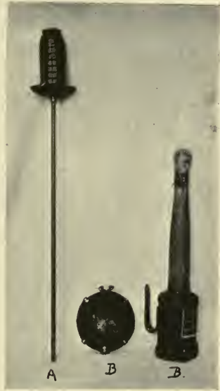
FIG. 8. Shows three types of grenade. A. Rifle grenade showing corrugations to aid in fragmentation. The long rod fits the barrel of the rifle and at bottom is a small revolving cap of copper which engages in the rifling. B shows two types of hand grenades, one on the right showing a hook for hanging on the belt.
