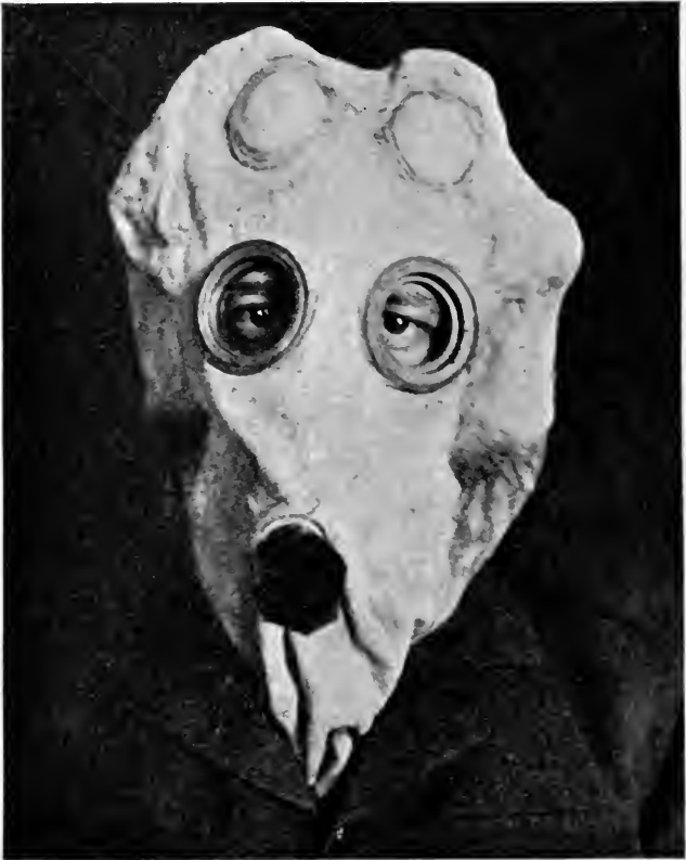
FIG. 151. Mask for use when a gas attack is being made. Mask is saturated with hyposulphite of soda and glycerine, which counteracts the effects of the gas.
