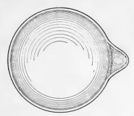
The dishes are conveniently heated in an oblong copper bath, with round holes cut in the top to receive them. The bath should be some six inches deep, and is charged with water. It is conveniently supported on a tripod, and heated with a Bunsen burner.
