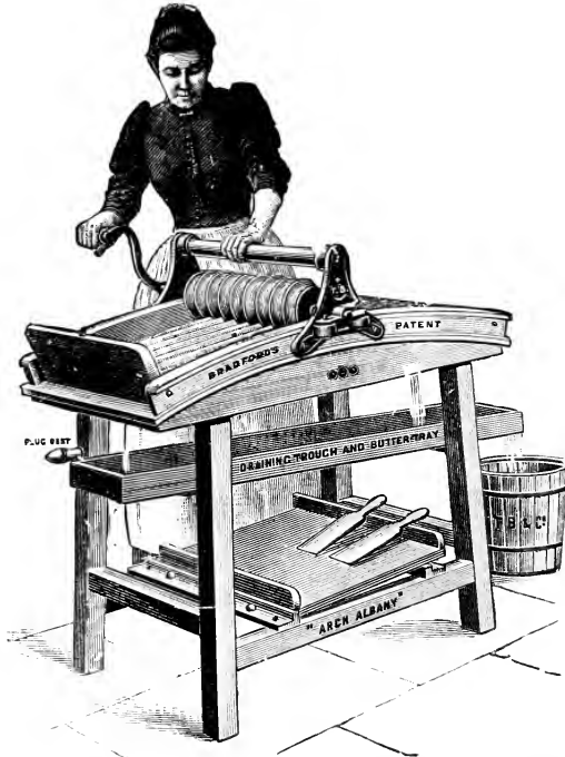
Fig. 40. BRADFORD'S "ARCH ALBANY" BUTTER WORKER Helicoidal Action and Double Drainage
