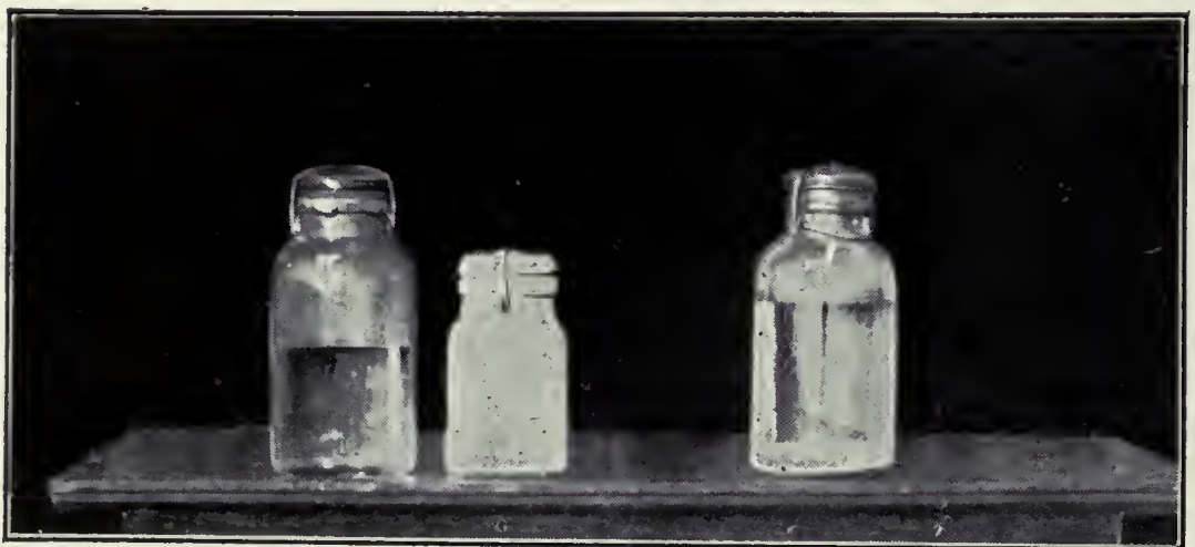
Figure 14—From left to right is sugar solution, slaked lime, viscogen. Note sediment of undissolved lime in bottle of viscogen at right
