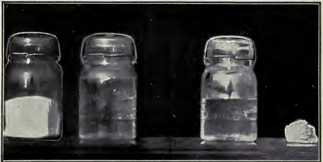
Figure 13—Materials for viscogen. At the left is sugar and water in which it is to be dissolved; at the right is lime and water in which it is to be dissolved
