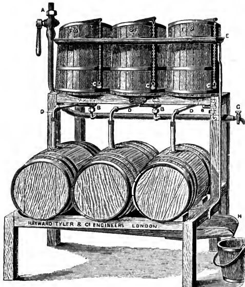
FIG. 107.—Apparatus for Filling Casks with Ginger Beer.
