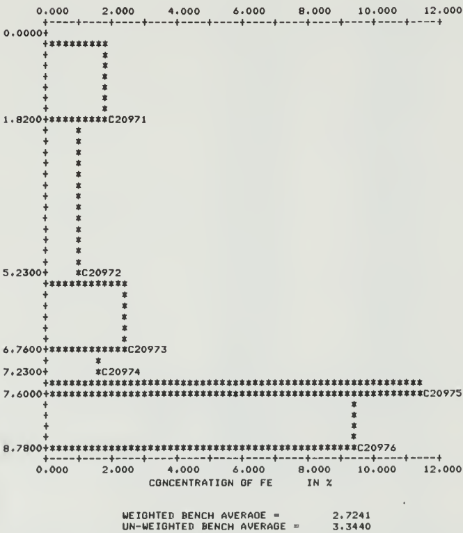
FIGURE VI-3. Bench set profiles for pyrite, Fe, As, and Pb from bench set B7.
