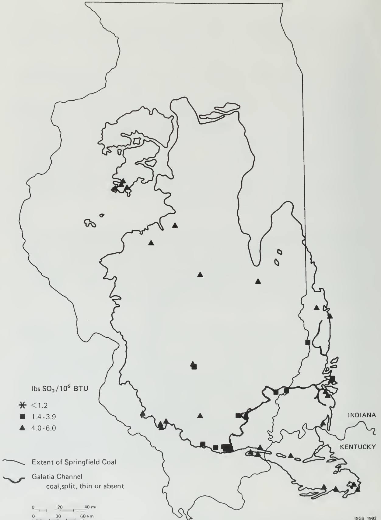
FIGURE VIII-2. Distribution of sulfur in the Springfield Coal expressed in pounds SO 2 per million Btu adjusted to a washed (estimated, laboratory) coal basis.
