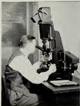
Special high-powered microscopes reveal details of the structure of clays and enable Survey scientists to predict their behavior and to discover new uses for them.
