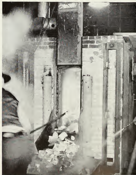
Pulling a charge of coke from the Survey's experimental oven.
