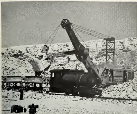
Loading limestone in a large Illinois quarry for the production of concrete aggregate, road material, agricultural limestone, and other purposes.
