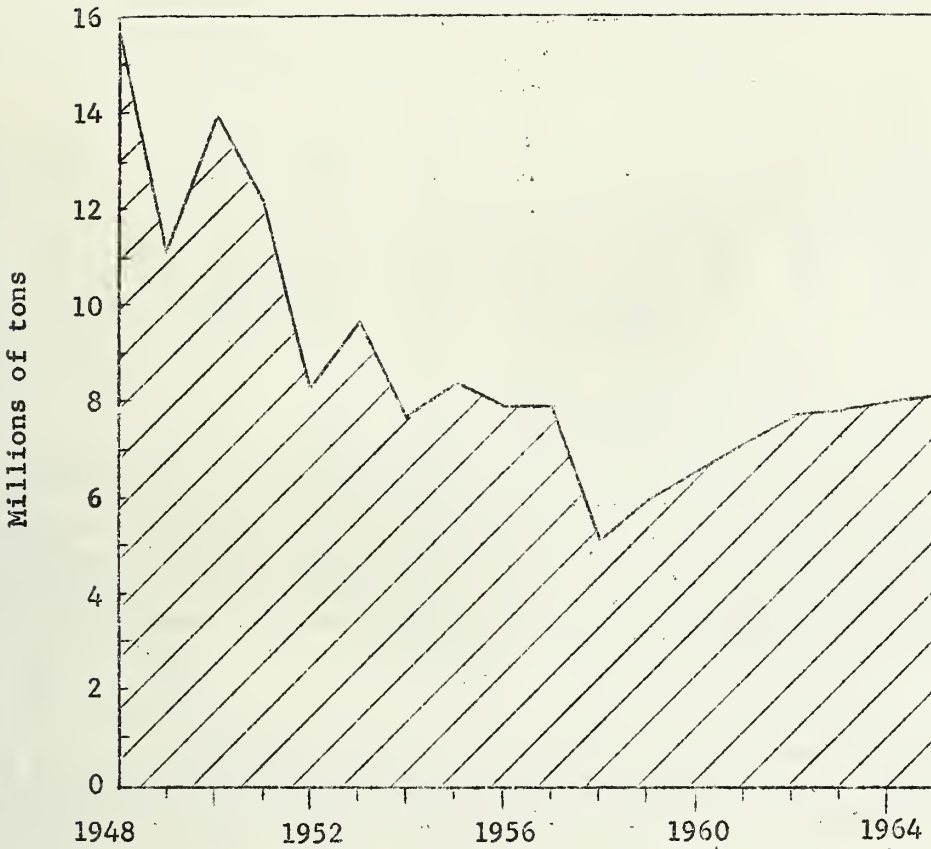
Fig. 7 - Annual coal production in the Springfield Region, 1948 to 1965. Practically all of the production came from underground mines; less than 1 percent was strip mined.
