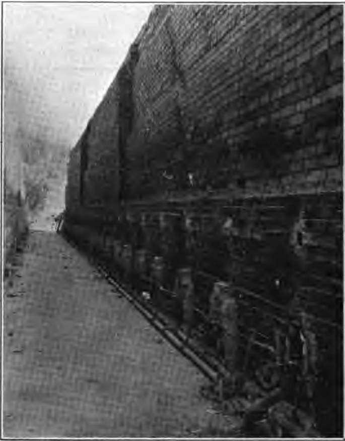
Photo No. 28. Crude oil burners for brick kiln, Craycroft-Herrold Brick Company, Fresno County.
