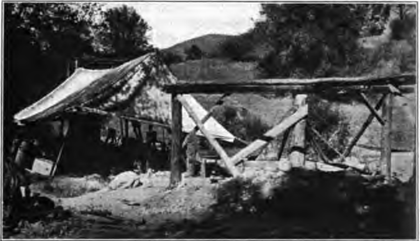
Photo No. 80. Arrastra and plant at Providence Mine, Temperance Flat, Fresno County.
