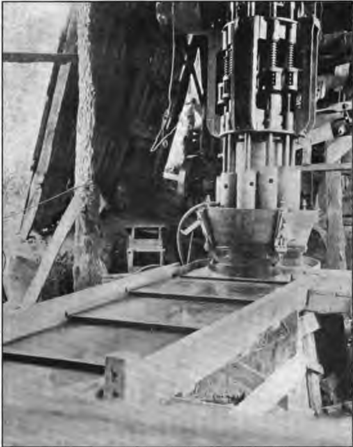
Photo No. 36. Straub patent mill (ten 175-pound stamps) at Contact Mine, Fresno County.
