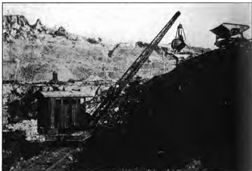
Photo No. 63. Orange-peel bucket excavator in quarry of Pacific Portland Cement Company, Solano County.
