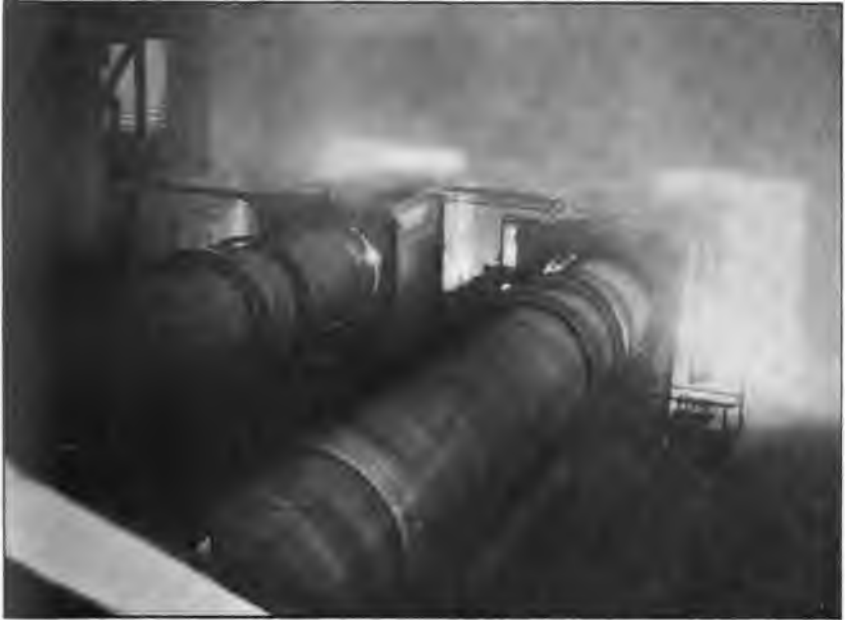
Photo No. 47. Rotary driers in mill of Standard Portland Cement Company, Napa Junction, Napa County.
