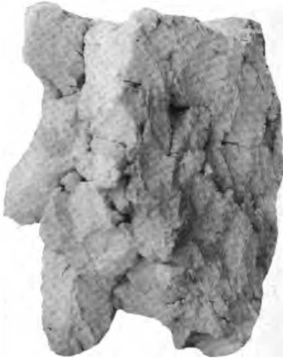
Photo No. 179. Magnesite from "Red Slide" deposit—Sonoma Magnesite Company, Sonoma County, California. Showing parallel shrinkage cracks. Two thirds natural size.
