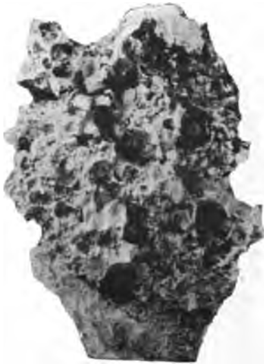
Photo No. 178. Magnesite from Kolling deposit, Sonoma County, California, showing pitted surface due to weathering. Two thirds natural size.
