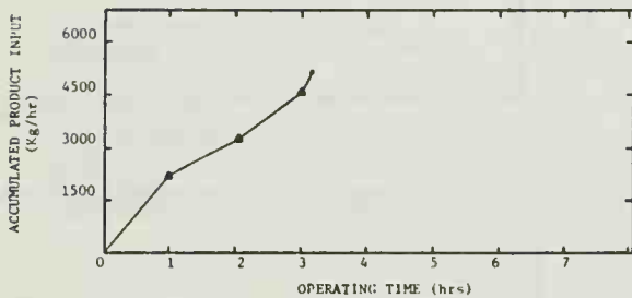
Figure A-24: Accumulated product input vs. operating time, Trial 3, Spring 1976, when processing spinach with conventional washers, west line.
