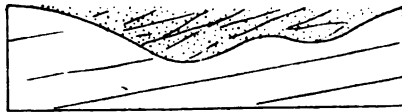
FIG. 3.—DIAGRAM SHEWING THE SAND FILLING THE IRREGULARITIES OF THE FLOOR BENEATH IT.
