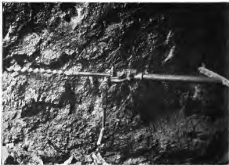
FIG. 14.—HARDY ROTARY DRILLING-MACHINE.
