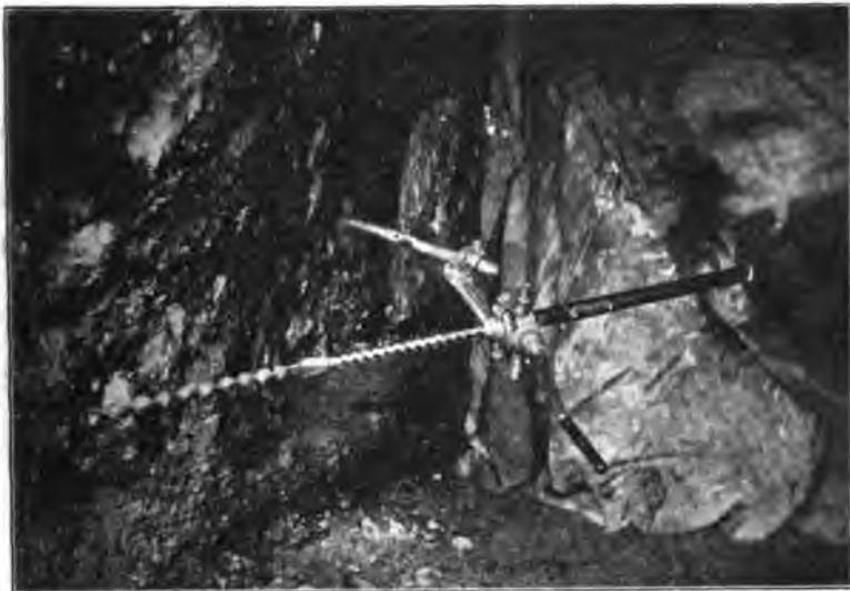
FIG. 13.—BLAKETT-HUTTON ROTARY DRILLING-MACHINE.
