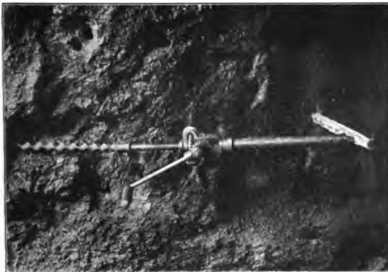
FIG. 15.—LIVINGSTONE ROTARY DRILLING-MACHINE.
