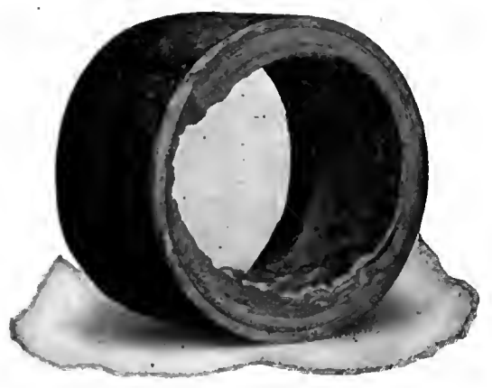
SECTION OF TUBE FROM A BADLY SCALED BOILER.
