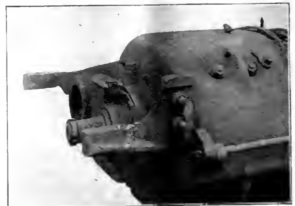
FIG. 6. GEAR CASE SUSPENSION LUG WELDED AND READY FOR USE.
