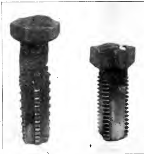
FIG. 4. BROKEN TAPS REMOVED BY ARC WELDING EQUIPMENT.
