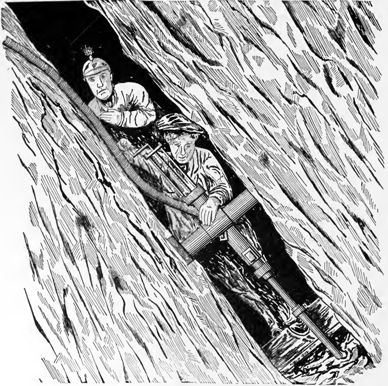
FIG. 7.—An 18-inch Stope in the Rand Mines, South Africa.
