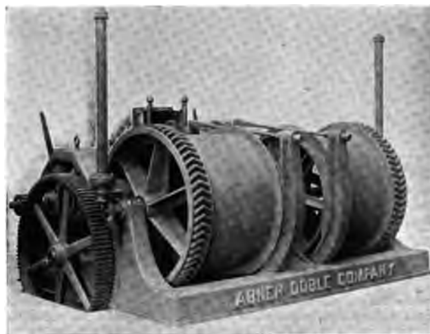
REAR VIEW OF THE GOTTSCHALK HOIST.
