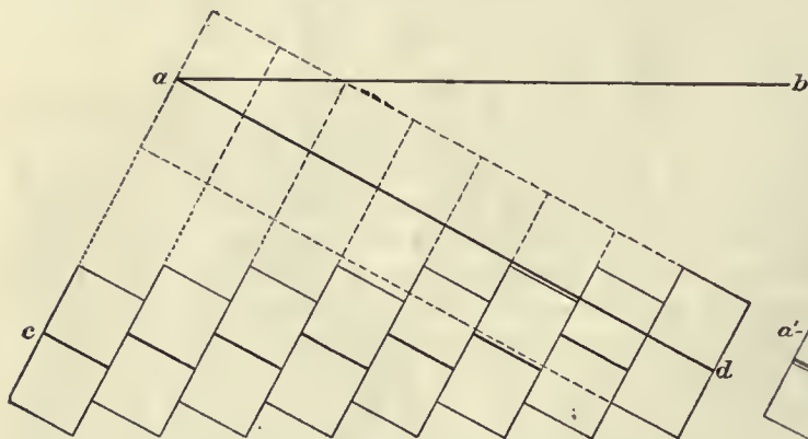
Fig. 4. Diagram illustrating tilting before faulting; vertical section at right angles to the strike of the faults. The original horizontal flow ab is tilted to ad and then faulted to cd .
