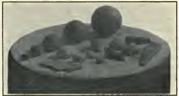
Balls, Stone, and Pieces of Steel From Ball-Mill.
