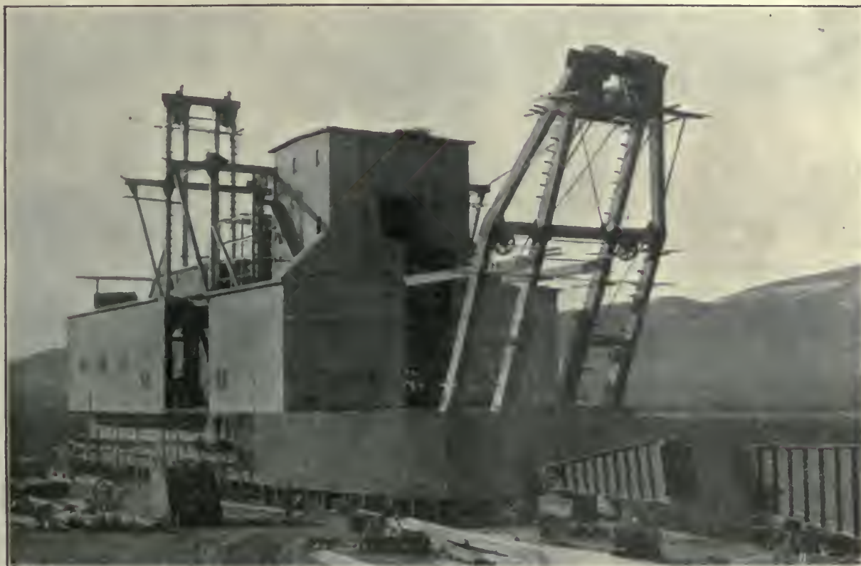
Dredge No. 2 Canadian Klondike M. Co., Near Dawson, Y. T. (Built by Marion Steam Shovel Co)
