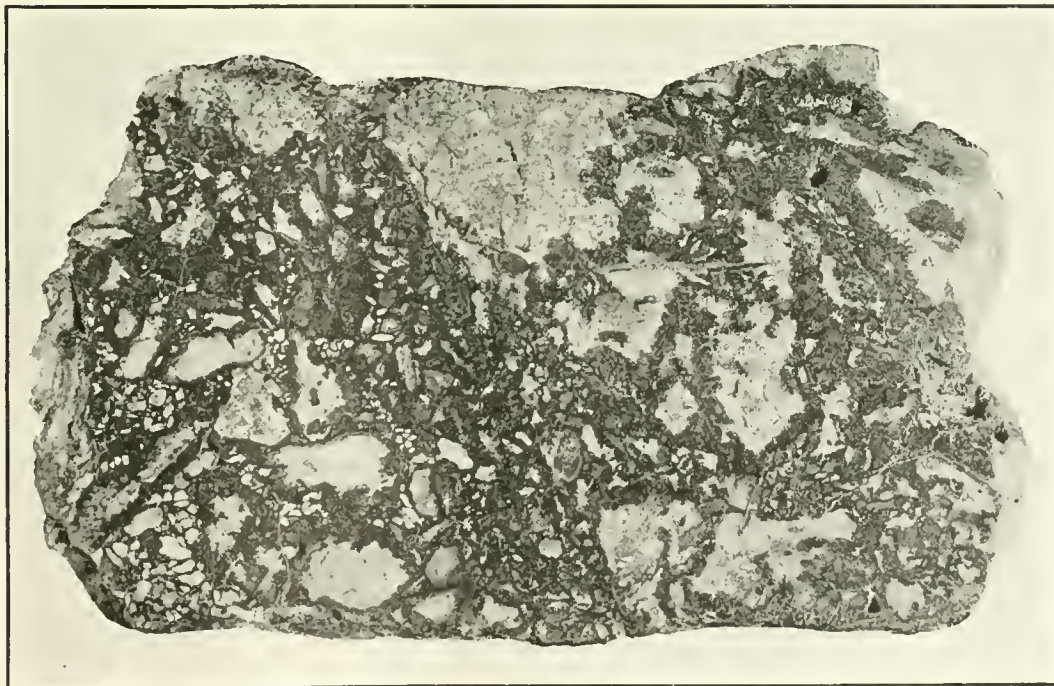
FERBERITE ENCLOSING FINELY BRECCIATED GRANITE. (By of U. S. Geological Survey.)
