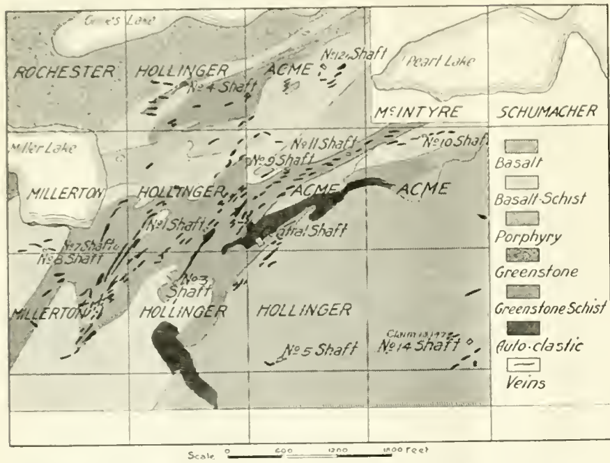
PLAN SHOWING VEIN OUTCROPS AND SURFACE GEOLOGY OF THE NEW CONSOLIDATION AT PORCUPINE, ONTARIO; THE HOLLINGER CONSOLIDATED GOLD MINES, LTD.
