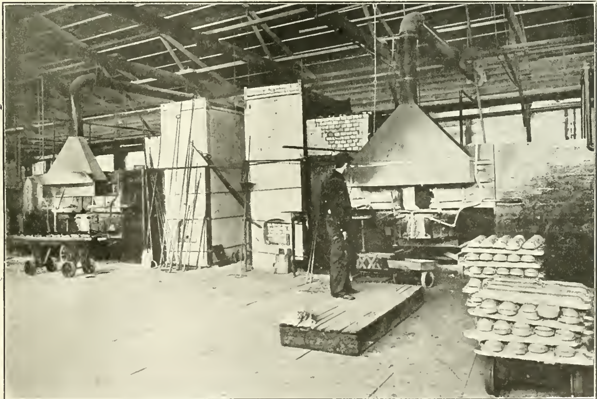
CUPELLATION FURNACES, WHERE THE LEAD, AS LITHARGE, IS REMOVED FROM THE GOLD AND SILVER.
