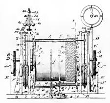
In a hoist, the combination of a substantially constantspeed motor, a driving or power shaft continuously driven to one direction from said motor at substantially constant
