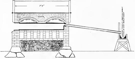
Fig. 1.—Retort Furnace for Quicksilver Ore. Cross-section.
