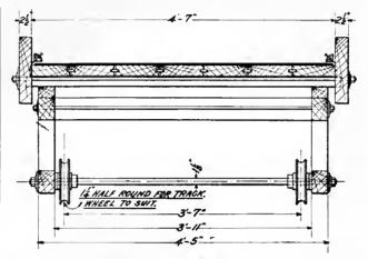
Fig. 2.-Cross-Section of Amalgamation Table.
