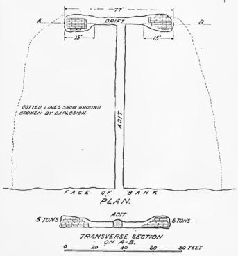
Fig. 4. Method of Blasting.
