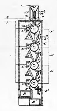
heat the material before it reaches the electrode, and means to maintain a heated atmosphere about the electrode into contact with which the material is delivered.
