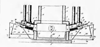
The method herein described of producing metallic copper directly from copper matte, which consists in subjecting the matte, while in hard condition, and in the presence of a flux, to the melting action of the flame of a burning mixture of oil-vapor, steam, and air.
