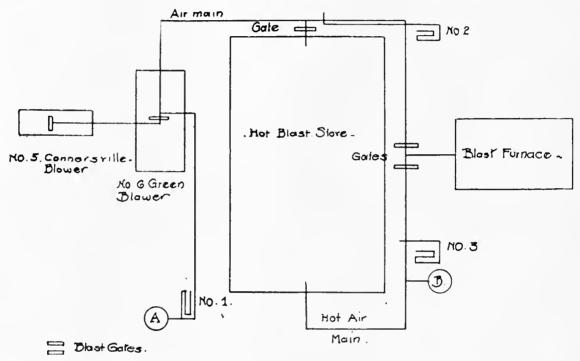
No. 1 and 2. Syphon Pressure Gauges. No. 3. Open Pressure Gauge.
