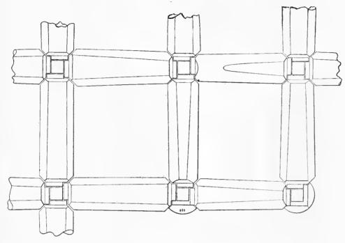
Fig. 2. Plan of Framing. Round Timbers.
