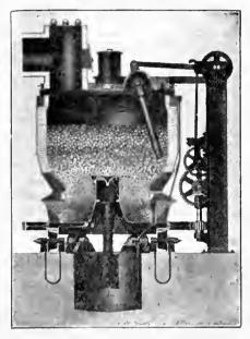
Sectional View of Hughes Patent Mechanically Poked Continuous
