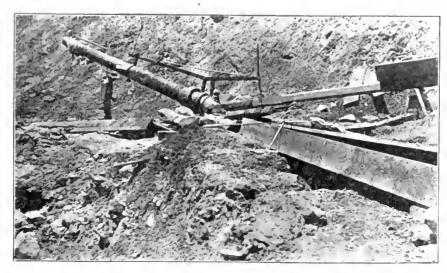
Fig. 5. Seven-inch Monitor at the Spring Valley Hydraulic Mine.
