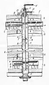
In a rabble apparatus, a hollow shaft and hollow arms therefor, a feeder passing centrally through the shaft and discharging a cooling medium thereinto at one end of the shaft, and means for circulating said medium through the shaft and arms vertically in series, and radially through a multiple, substantially as set forth.
