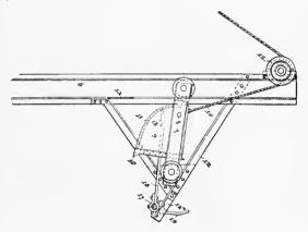
The combination with an excavator-bucket and means for effecting the inversion thereof, of a cleaner pivotally mounted externally of said bucket, said cleaner having an operating edge adapted to engage the forward edge of the bottom wall of the bucket and scrape over said bottom wall during the inverting of the bucket, substantially as described.
