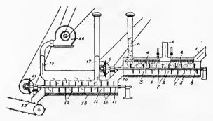
The process of making coal briquets consisting in, first, heating the pulverized coal; second, melting the organic binder separately therefrom; third, mixing both substances while hot; fourth, reducing the mixture to a granular, floury condition by continued mixing under an air-blast; and, fifth, supplying the same while floury and cool to the press to make briquets, substantially as described.
