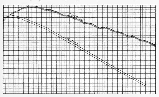
Fig. 2. Sectional Elevation Showing Relation of Slope to Surface.
