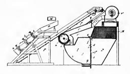
Apparatus for the manufacture of flake mica from mica plates, comprising one or more pairs of bending-rolls, means for conducting the mica plates between said rolls, a flaking-chamber provided with an intet-chute inclined to the length of said chamber, means for conveying loosened and partly-
