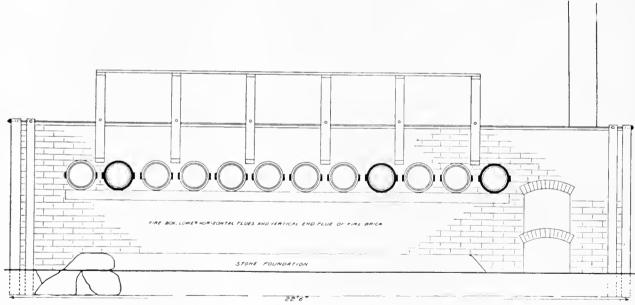
Fig. 2.—Retort Furnace for Quicksilver Ore. Front Elevation.
