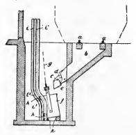
In an apparatus of the character described the combination with a chute and a vertically movable skip of guides for said skip standing at a distance from the end of the chute to permit the skip to clear the same in its movement and carried inward toward the vertical plane of the chute below the same to guide the skip below the end of the chute.
