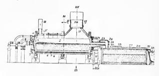
The method of extracting metal values from ores through liquation without carbonaeeous fuel, which eonsists in feeding silieious ore to a bath of molten matte in excess of the amount that will flux with the constituents of the bath, and eausing the excess portions of the ore to yield their values to the bath by liquation; substantially as described.
