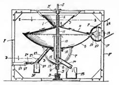
METALLURGICAL FURNACE.—No. 829,671; George W. Shear, Joliet, Illinois.
