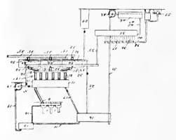
a series of settling-tanks communicating with each other, the eyanide-tanks, means for connecting said cyanide-tanks together, means for conveying the cyanide solution from the settling-tanks into the cyanide-tanks and from the cyanide-tanks again into the settling-tanks.
