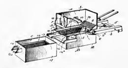
In an ore-slimer, the combination with a receptacle for dispensing ore tailing, of a series of slime-tilters made up of intermediate boxes having outlet openings in their walls, removable screens mounted within said walls, means for binding the screens in place, and an end filtering-box having liquid outlets in its walls and side and end inclined screens converging upwardly and arranged to intercept the liquids as they pass out of said end box.
