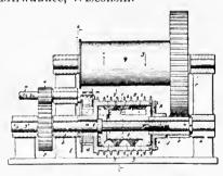
In an automatic load-brake the combination of a shaft having two expanding heads mounted thereon, one of said heads being movable axially toward and from the other, an expansible friction-ring between said heads, a shell surrounding said ring and free to turn in one direction, and means for holding said shell against turning in the opposite direction, substantially as described.
