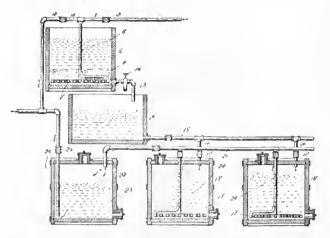
The herein-described leaching process consisting in placing suitably pulverized ore in a tank containing a solution composed of water, common salt, alkali-metal intrate and sulphurous acid, and subjecting the pulp thus formed to the action of air and steam simultaneously introduced.
