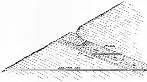
Method of Working Inclined Orebody.
