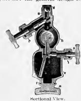
good. The cup was constructed not only with a view to proper and positive lubrication, but also to withstand severe service. The filling hole is large, which users will appreciate,
