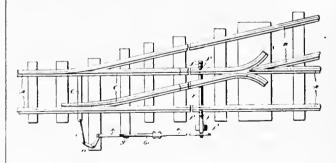
In a device of the character described, a main line, a siding, a switch, means for automatically operating said switch, including a single tripping device positioned beyond the heel of said switch and adapted to be engaged by a wheel of a car after passing over said switch to throw the same to connect the main line and siding, and means for locking said switch in its open and closed position.
