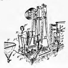
The process of separating powdered minerals from one another which consists in suspending the powdered minerals in a liquid, subjecting the mixture to a gas-pressure and thereafter relieving the pressure whereby bubbles of gas are liberated in the puip and carry certain minerals to the surface.
