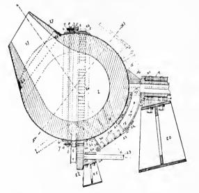
A converter for converting copper and other mattes and the like having formed in the lining thereof conduits arranged about a central axis, and opening upwardly through said lining and in a direction oblique to the plane through
