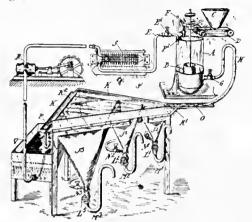
The herein-described process of concentrating ores which consists in mixing the powdered ore with water, adding a small proportion of an oily liquid having a preferential affinity for metalliferous matter (amounting to a fraction of one per cent on the ore), agitating the mixture until the oil-coated mineral matter forms into a froth, and separating the froth from the remainder by flotation.
