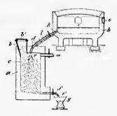
The described process which consists in bringing in contact with each other a compound or compounds of a metal or metals, an agent capable of generating metallic vapors from said compound or compounds, and an incandescent fluid heat-carrier, and leading off the vapors and gases for separation, substantially as described.
