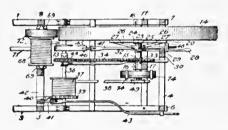
In a well-drilling machine provided with a drill, a cable attached to said drill, a spool for said cable, and means for paying out the eable from said spool; a drill-wheel carrying a sheave-wheel for engaging said cable to regulate the stroke of the drill, a ratchet-wheel for driving said drill-wheel, means for intermittently locking said drill-wheel and ratchet-wheel together for drilling purposes, and means for permanently locking said drill-wheel and said ratchet-wheel together.
