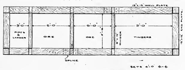
Fig. 1. Plan of Timber-set for Star-Pointer Shaft.
