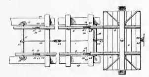
The combination with a cage in a shaft and a track leading thereto, of fore and rear carstops connected together and movable oppositely up and down through the track, to stop and release the first and successive cars respectively, a tripper in the shaft arranged to be struck by the cage, and operative connections located under the track and extending between the tripper and the stops, to raise and lower the latter.
