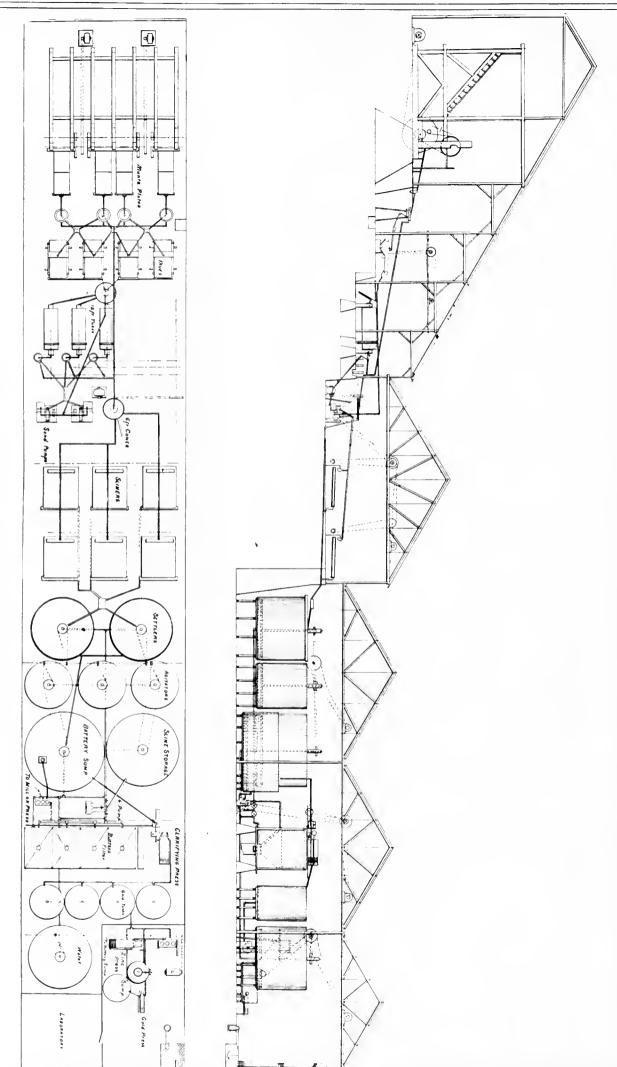
Plan and Elevation of a New Cyanide Plant.
