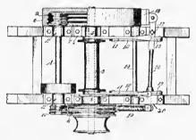
In hoisting apparatus, the combination of a drum having a plurality of frictional surfaces, a drive-shaft having a plurality of frictional surfaces, and means for shifting the drum relative to the shaft whereby one of the frictional surfaces thereof will engage one of the frictional surfaces of the drive-shaft and the other frictional surface of the drum will simultaneously disengage the like surface of the shaft.
