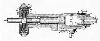
In a drill mechanism, a casing, a hollow drill-shank inserted in the casing and provided with a lateral opening, a cylinder formed within the casing adjacent the shank, a hollow piston mounted to reciprocate within the cylinder, an elastic packing carried by the piston and in contact with the shank, a duct forming communication between the casing and the cylinder and opening in the rear of the piston, and means to admit fluid under pressure to the casing.
