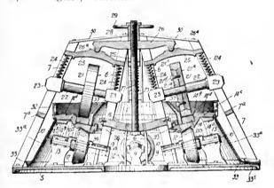
The combination in a pulverizing-mill, of an outer and inner series of posts, an annular revoluble mortar located between said series of posts, rollers supporting the same, means for rotating the mortar, and annular mortar-centering rings carried respectively by the mortar and the inner series of posts, said rings having opposing edges in the surface of a right cone concentric with the mortar-axis.
