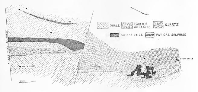
Fig. 6. Plan of Second Level of Esperanza Mine.
