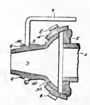
The combination with the nozzle of a hydraulic mining apparatus, of a tubular deflector having a swinging connection with the nozzle and provided with external projections, and a controlling handle having a loop embracing the deflector back of the projections, the loop being provided with internal seats capable of alinement with the projections to permit application and removal of the loop.
