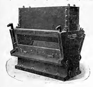
the faces where the sections are joined are machine-planed so perfectly as to make a precise fit. This gives the mortar a neat symmetrical appearance when set up, making it as solid and serviceable as are those not sectionalized. The mortar is arranged for inside amalgation, and a splash-plate may be attached to the lip if desired. No piece weighs more than 300 lb. In like manner, the entire milling plant may be built in similar sections where mule-back transportation is required.
