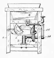
In an ore-feeder, the combination of a rotatable feed-table, of a rock-shaft, of a gear loose on said shaft engaging the feed-table, of means secured to the said shaft for frictionally engaging with the gear to actuate the same with the movement of the rock-shaft, and cam-actuated devices for imparting motion to the said rock-shaft.
