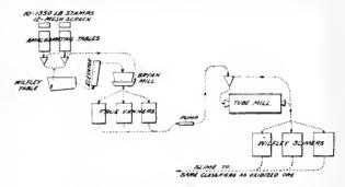
Fig. 4.—Treatment of Sulphide Ore.
