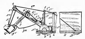
A bottomless pneumatic shield provided interiorly with means whereby foundations may be constructed on or in the bed of a river from within said shield, with means for keeping said shield under water, and with means for advancing the shield horizontally as the foundations therebelow are constructed.
