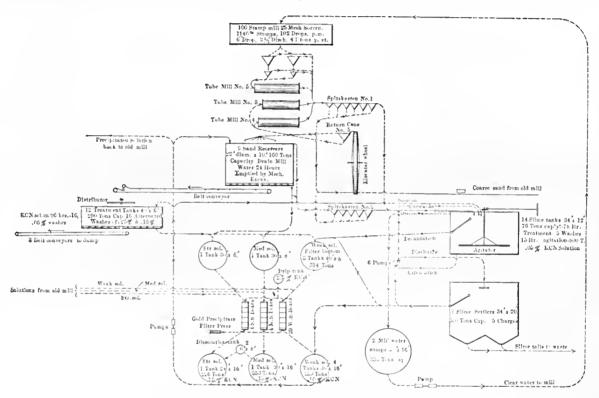
Fig. 1.—Diagram of Cyanide Treatment at Plant No. 2. (September, 1905.)
