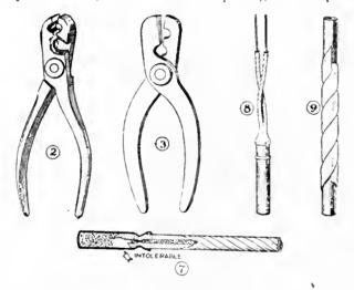
into the same caps which had failed before, but crimping them with a broad-faced tool, every one has exploded. Hence, to avoid choking the fire in the fuse, always see that the fuse is pushed down into the cap as far as the composition and secured to the cap with a broad tool, making the flat compression around the shell. (Fig. 5) Avoid thin crimpers, which make a groove around the shell. (Fig. 4)
