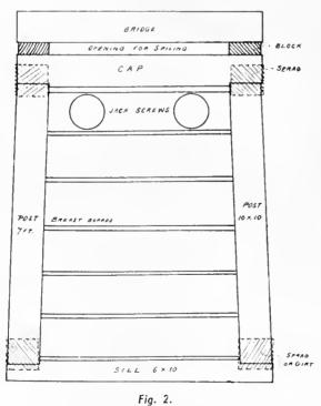
it back. Therefore, two jack-screws are brought to the spot and they are placed with heel (or base) on a cross-timber carried by the rear set. The top breast-board is now advanced 8 or 12 inches and a sawed-off block is inserted within the space thus obtained; this block holds the breast-board in its advanced position. The next board is pushed to a corresponding position, as before, cleaning
