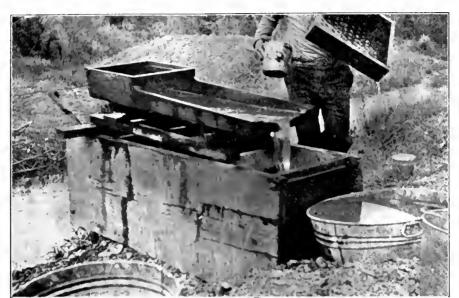
Rocker and Second Settling Vat at Central Dredging Company's Drilling Plant.
