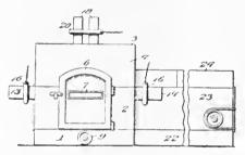
An electric furnace comprising a furnace proper, horizontally-arranged conductors extending through opposite walls of the furnace, a resistor supported by the inner ends of said conductors, and a conductor supported by the furnace and movable in a plane at right angles to the plane of the first-mentioned conductors.
