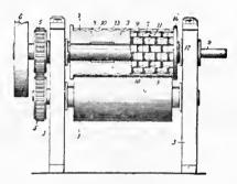
A crushing-roll having teeth formed in straight rows extending longitudinally of said roll, and having straight webs lying between said rows and extending longitudinally thereof.
