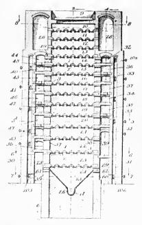
The process of treating materials by the aid of heat, which consists in eausing the material and the heating medium to travel from the cooler part of the apparatus to a hotter part thereof at rates of travel independent of each other, substantially as described.
