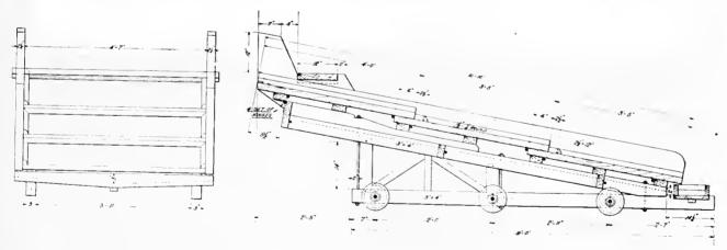
Fig. 3.-Movable Amalgamation Table Used in the Combination Mill.
