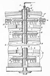
In a furnace having a plurality of hearths, a hollow shaft passing through the hearths, a series of hollow arms radiating from said shaft and extending into the several hearths, parting motion to the said rock-shaft.
