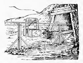
A monotrack-tramway comprising uprights having their upper ends split and expanded to form sockets, and a rail of substantially arrow form in cross-section having its body fitting in the split portions of said uprights.
