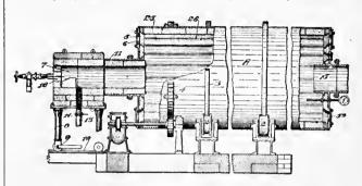
The combination with a revoluble ore-roasting shell having means whereby ore may be admitted thereto, of a combustion-chamber separate from the shell and movable toward and from the inlet end thereof said chamber having an opening in one end for the admission of a gaseous fluid and having an air-supply pipe fixed to and movable in unison with it.
