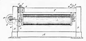
An improved ore-concentrator consisting of a main frame having vertical end standards, transverse beams connecting the upper portions of said standards, an independent frame within said main frame below the top of the standards, an endless belt operable in the independent frame, boxes in the upper portions of said standards, an independent frame, boxes is continuously decomposed and regenerated until all the free acid has become neutralized substantially as set forth.
