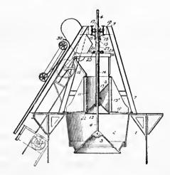
In a furnace-charging mechanism the combination with a receiving-chamber communicating with the interior of the furnace, of a distributing-bell adapted to close the lower end of said chamber and constructed to accumulate the stock delivered to the chamber to one side of the same when the bell is in closed position, means for opening the distributing-bell to discharge the contents of the chamber, and means for shifting the position of the bell to vary the point of discharge.
