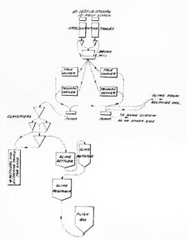
Fig. 1.-Treatment of Oxidized Ore.
