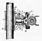
In a rock-drill, in combination, a supporting column, a sleeve mounted on the column, a trunnion carried by the sleeve, a drill-cradle having a hub fitting over the trunnion, a worm-gear formed on the hub, and a worm-shaft journaled on the sleeve and meshing with the worm-gear.
