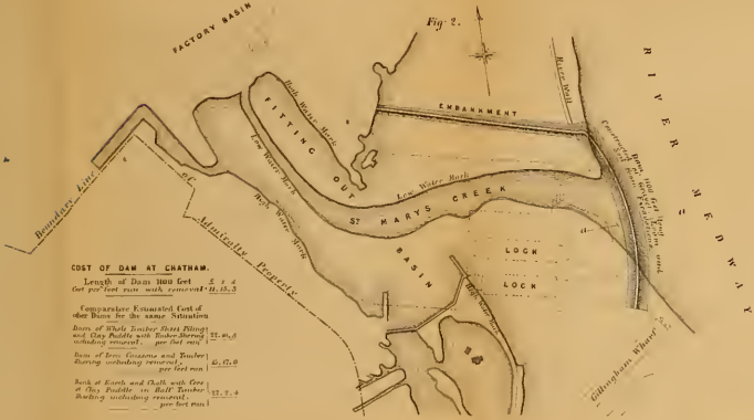
PLAN SHEWING POSITION OF DAM ACROSS THE MOUTH OF ST MARYS' CREEK.
