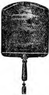
Fig. 1. The Audiphone in its natural position; used as a fan.
