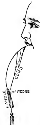
Fig. 3. The Audiphone properly adjusted to the upper teeth; ready for use. (Side view.)
