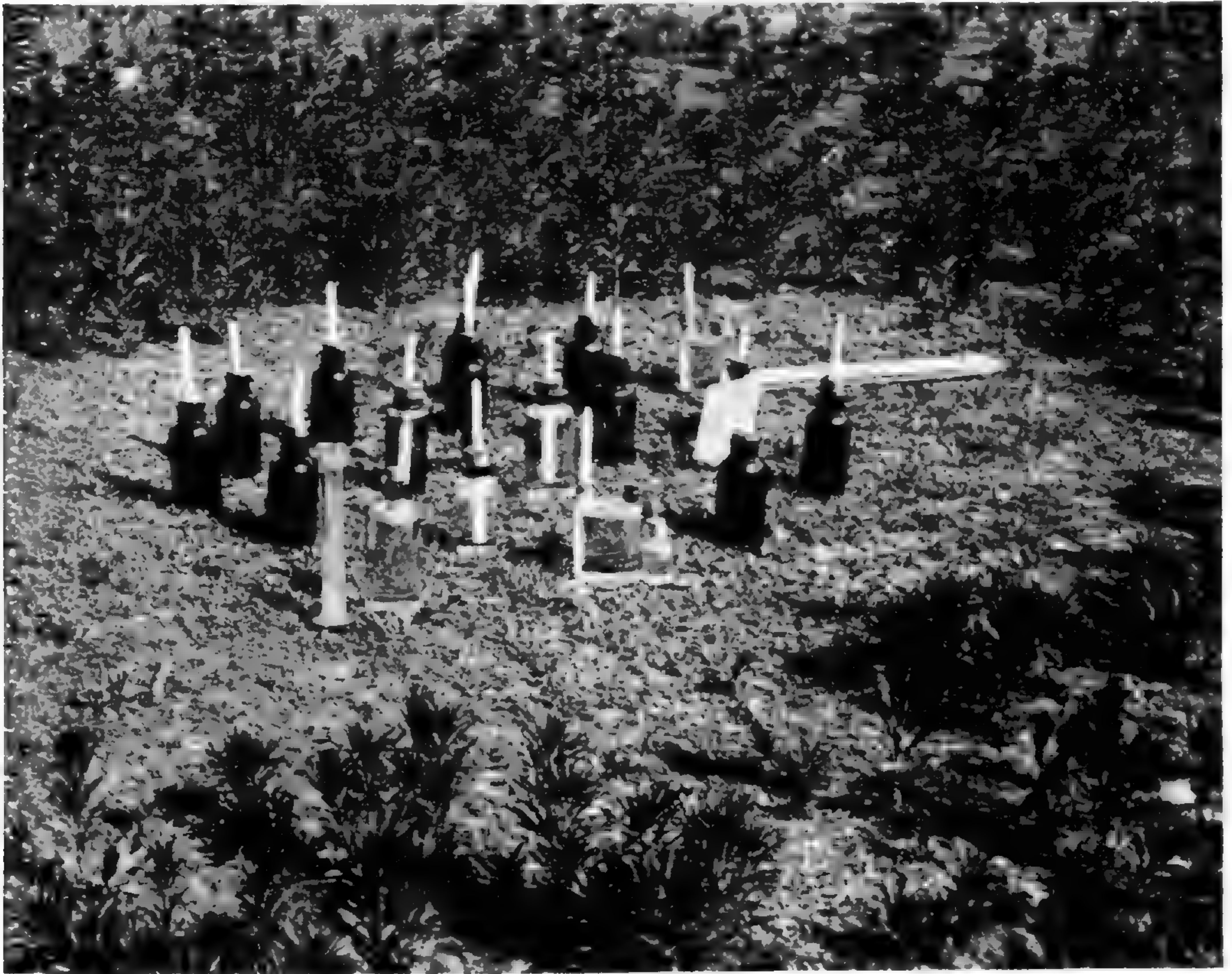
FIG. 1.—Atmometers in process of standardization, June 22, 1910; photograph by F. C. GATES.
