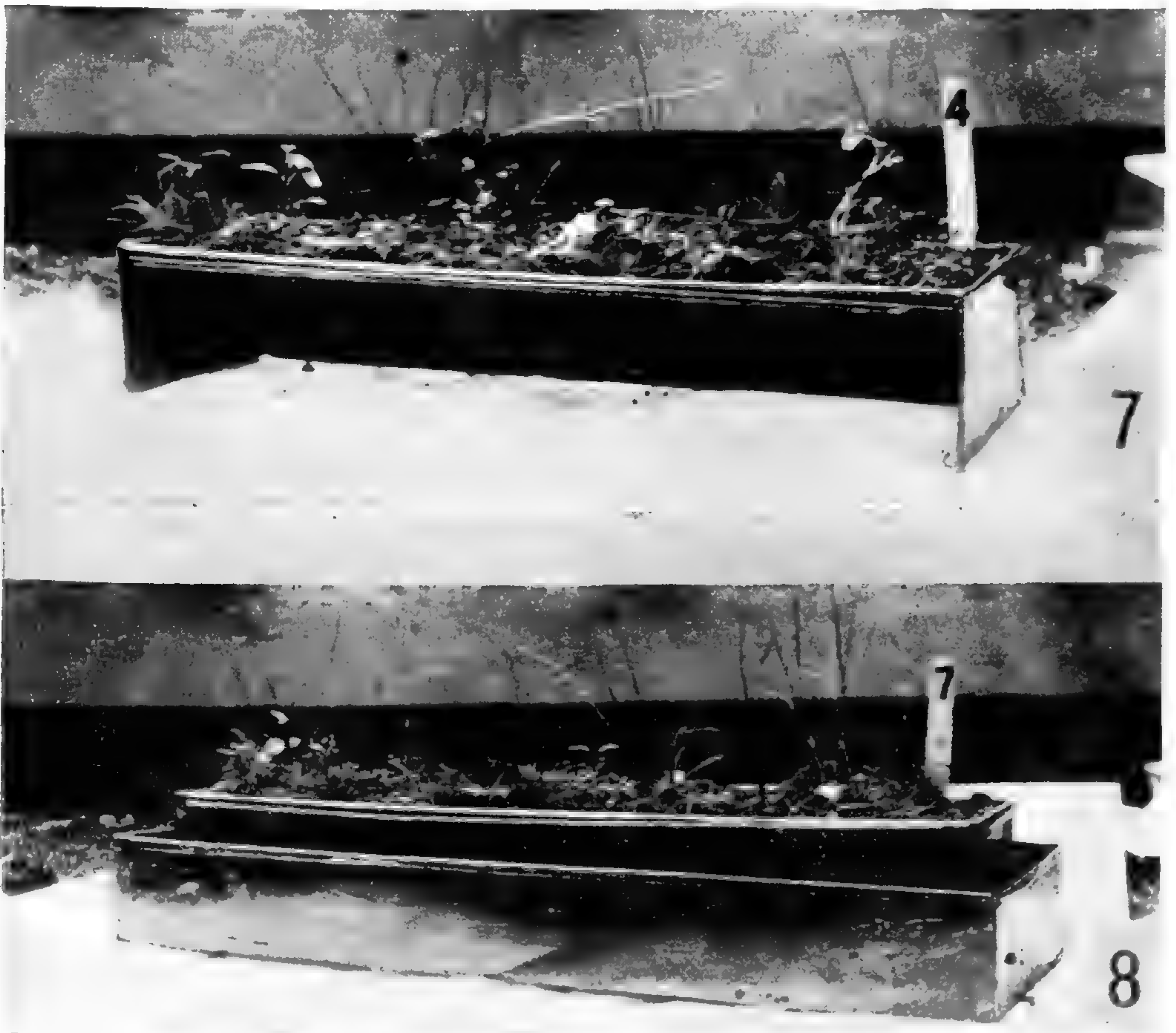
FIGS. 7, 8.—Growing boxes used in experimental work: fig. 7, growing box with diagonal glass side facing camera (removable sheet iron false side is in place covering glass); fig. 8, growing box similar to that in fig. 7 placed in pan containing water, thus maintaining fixed water level in growing box.
