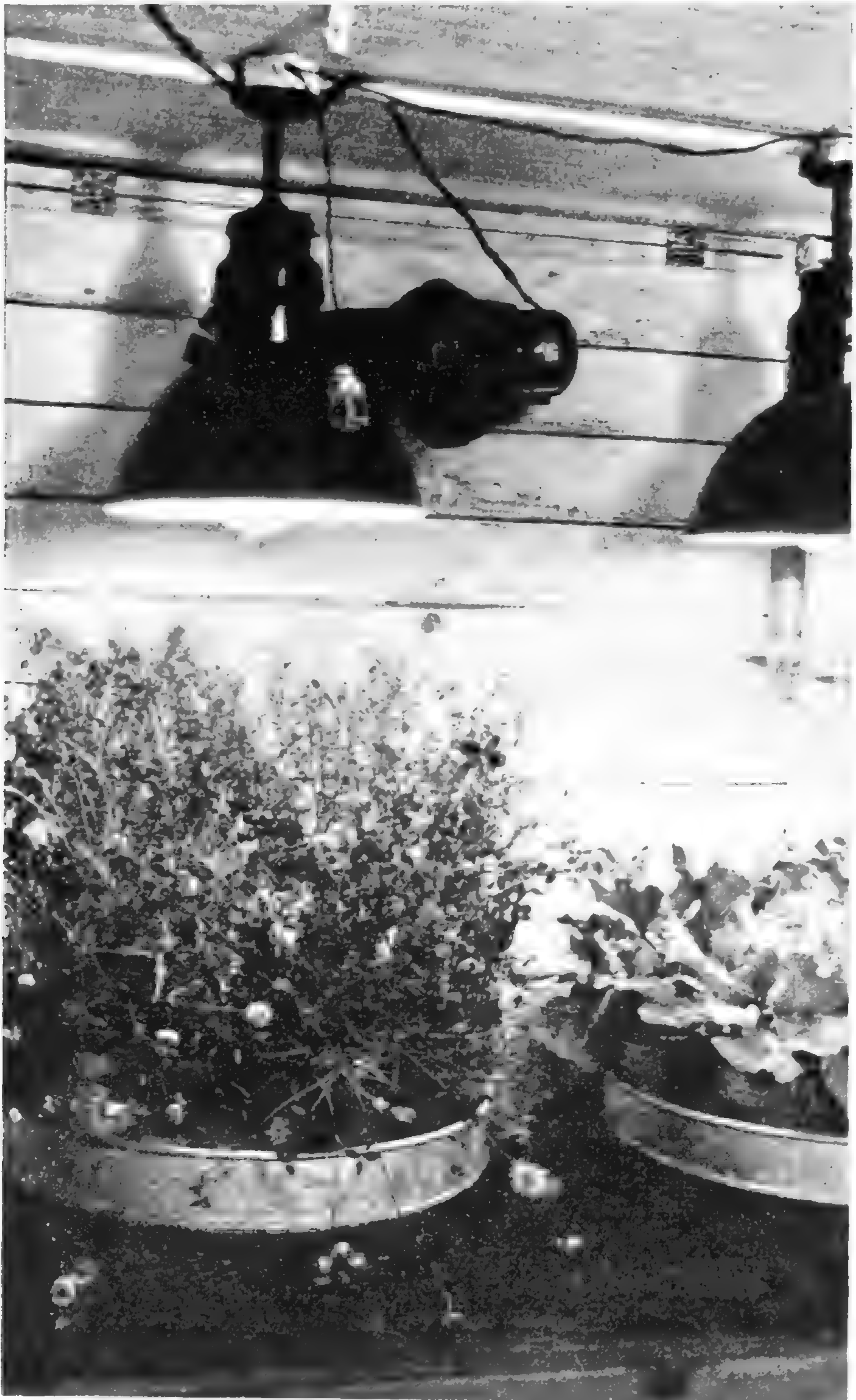
FIG. 2.—Rotating tables operated by electric phonograph motor to equalize light and temperature.
