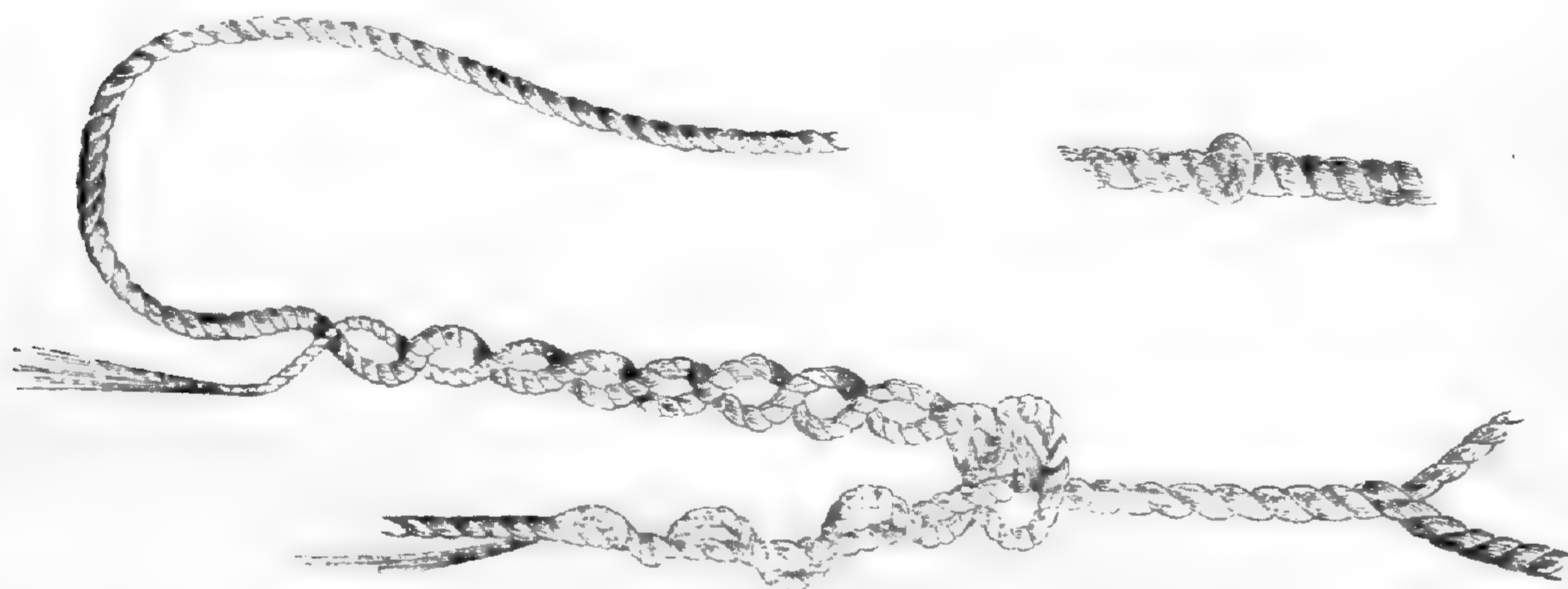
Fig. 3. Sketch illustrating method of preparing fine cord and fishing lines from oil-palm fibre.
