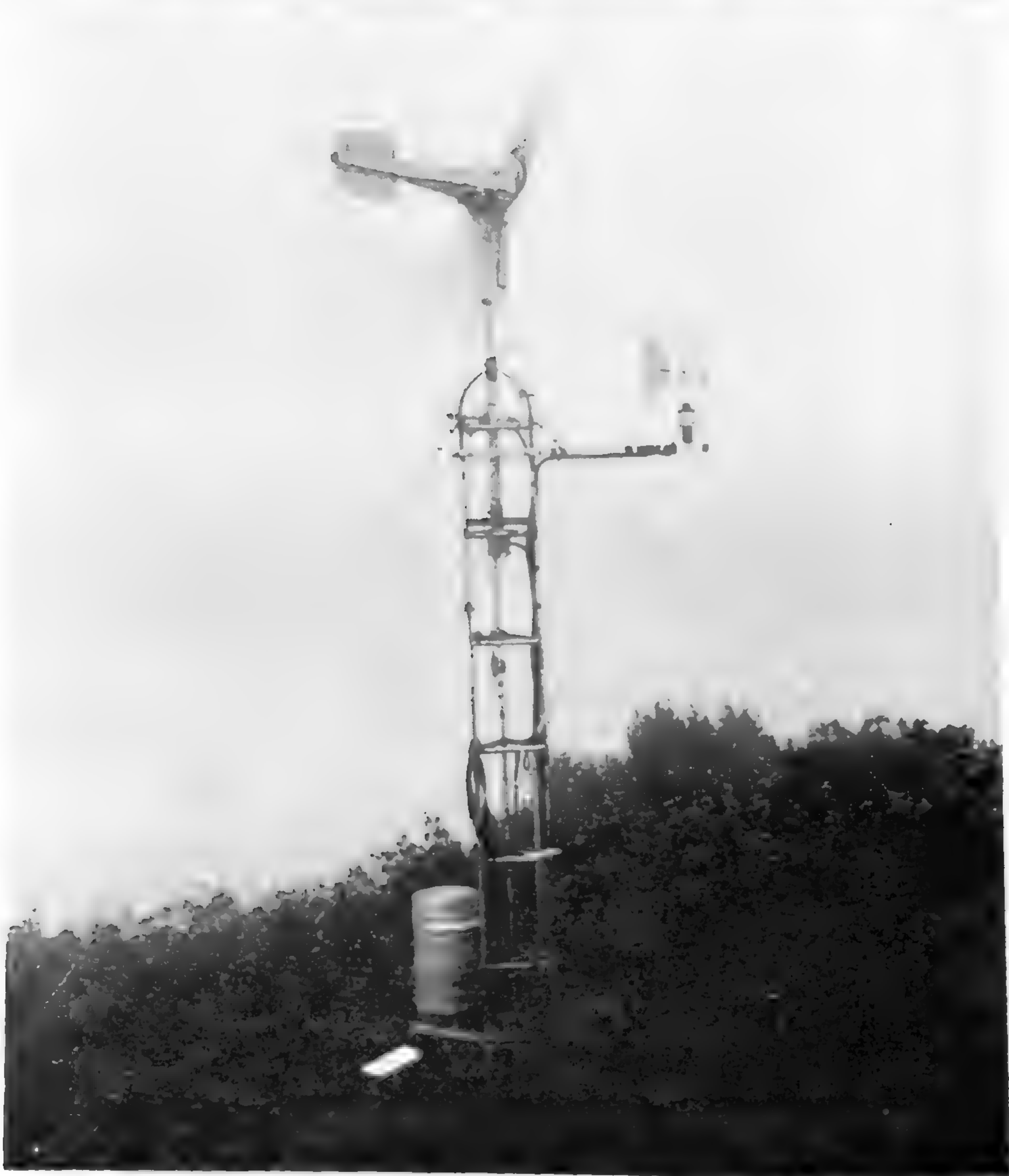
ABOVE: FIG. 1. Thermometer shelter just above canopy.
