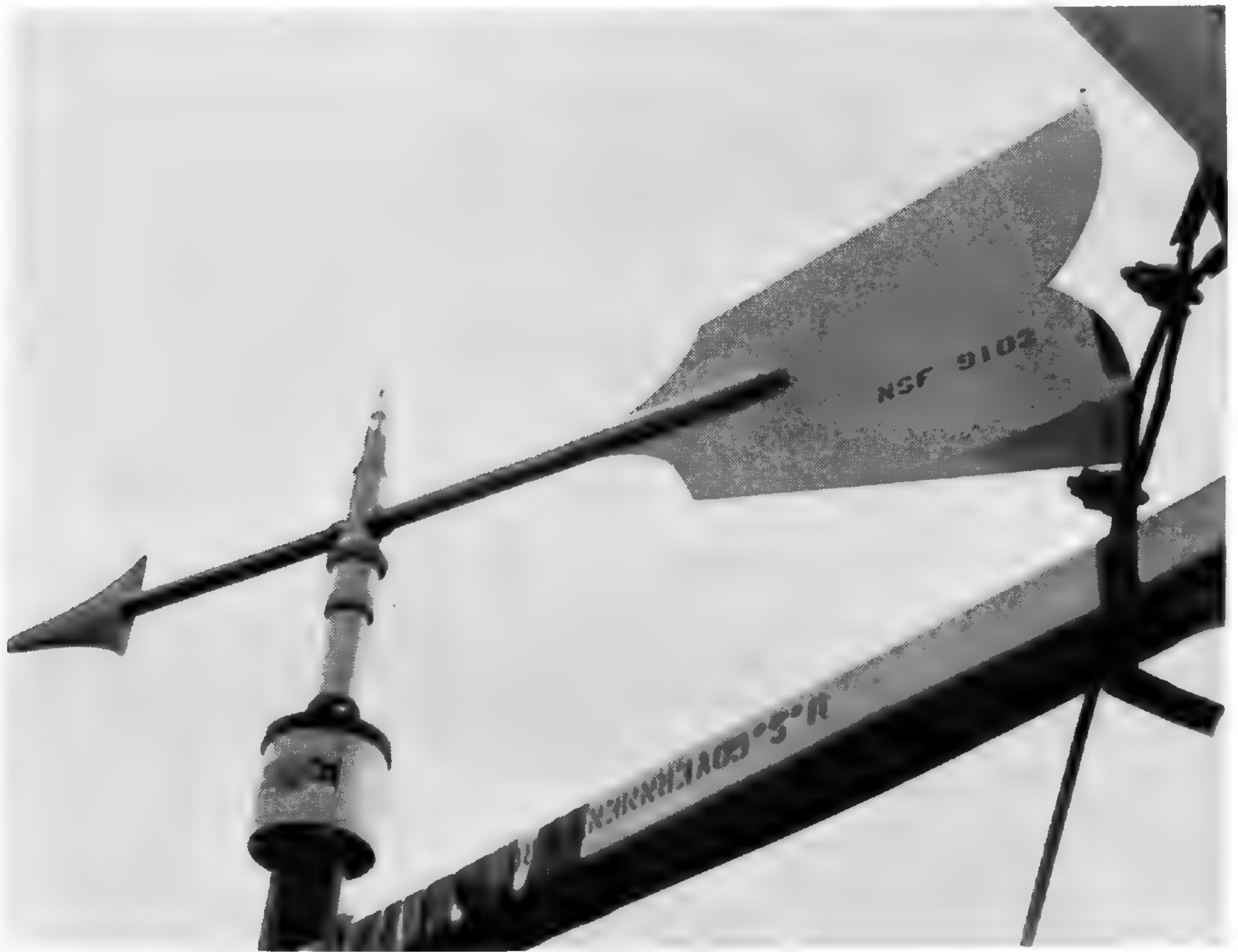
FIG. 8. Wind vane on top of tower.
