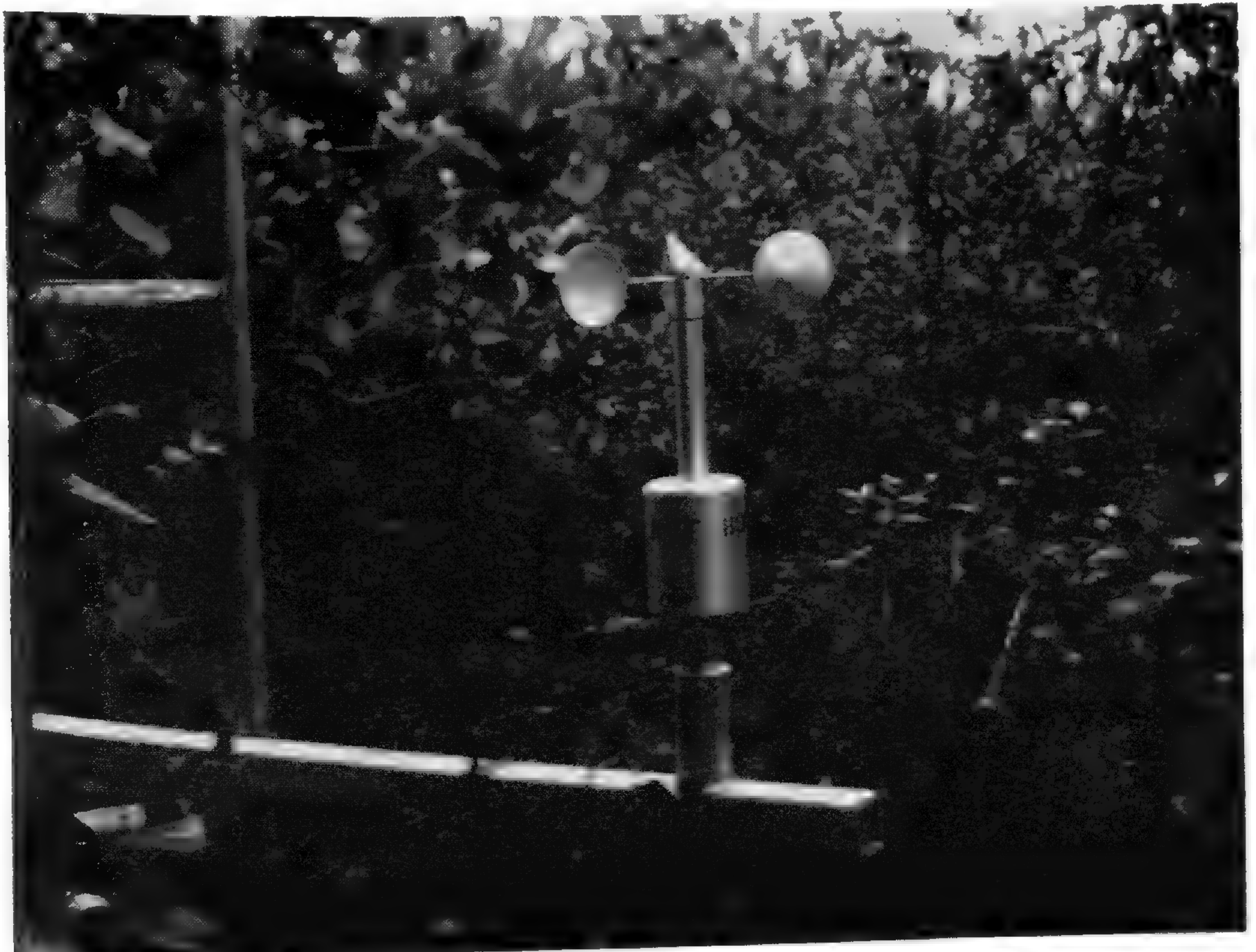
FIG. 7. 3-cup anemometer used for measuring wind speed below the canopy.
