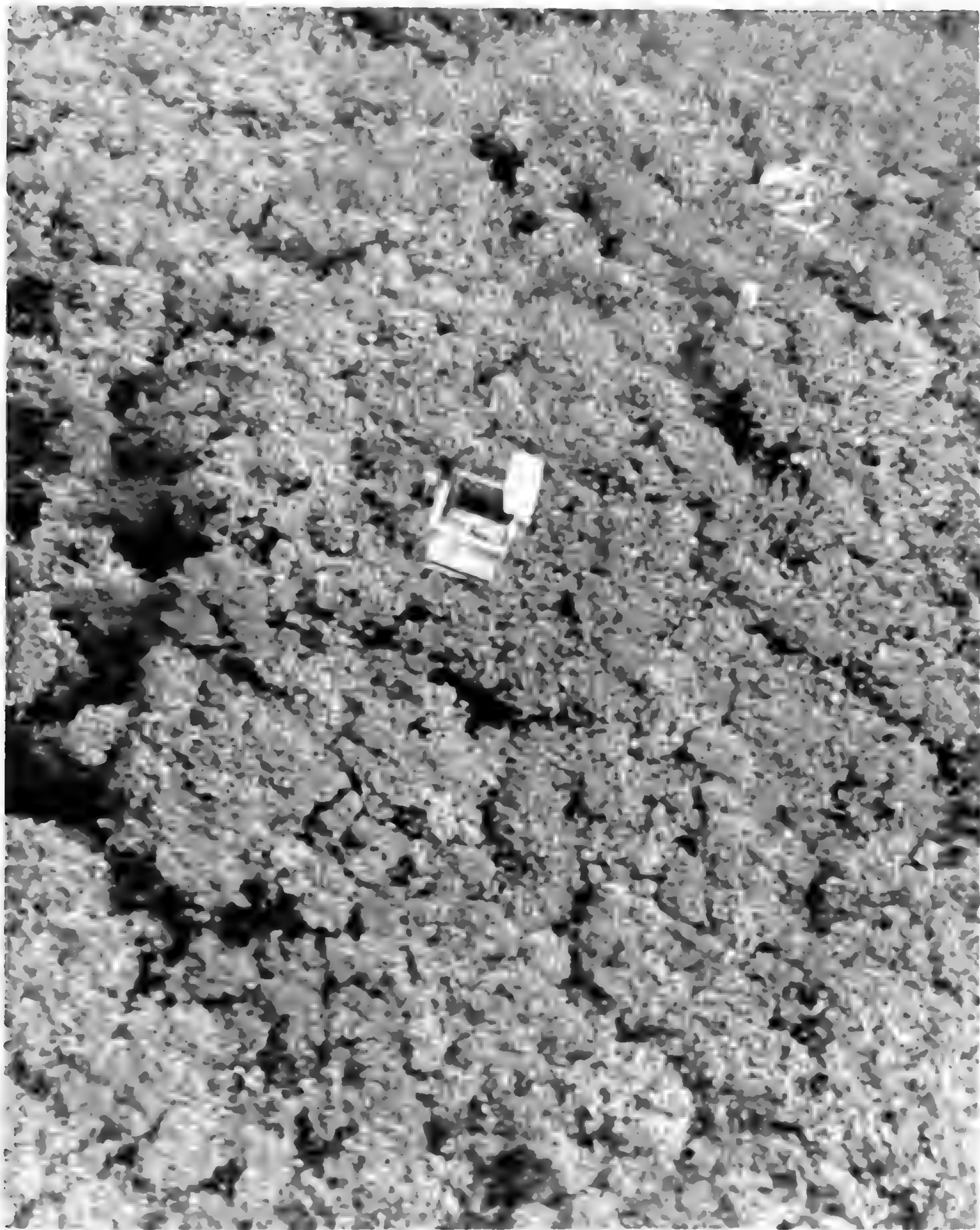
FIG. 13.—An aerial view of the study site on the summit of Pico del Oeste. The platform on top of the observation hut holds the instrument shelter. Adjacent are two Durham pollen samplers. The linear board on the floor points due north. The tower holds a wind generator, recording rain gauge, two anemometers and a wind direction indicator. White markers on bamboo poles are visible and were used to correlate ground and canopy studies of the vegetation. Photo reproduced from a color negative, courtesy of the U. S. Army.
