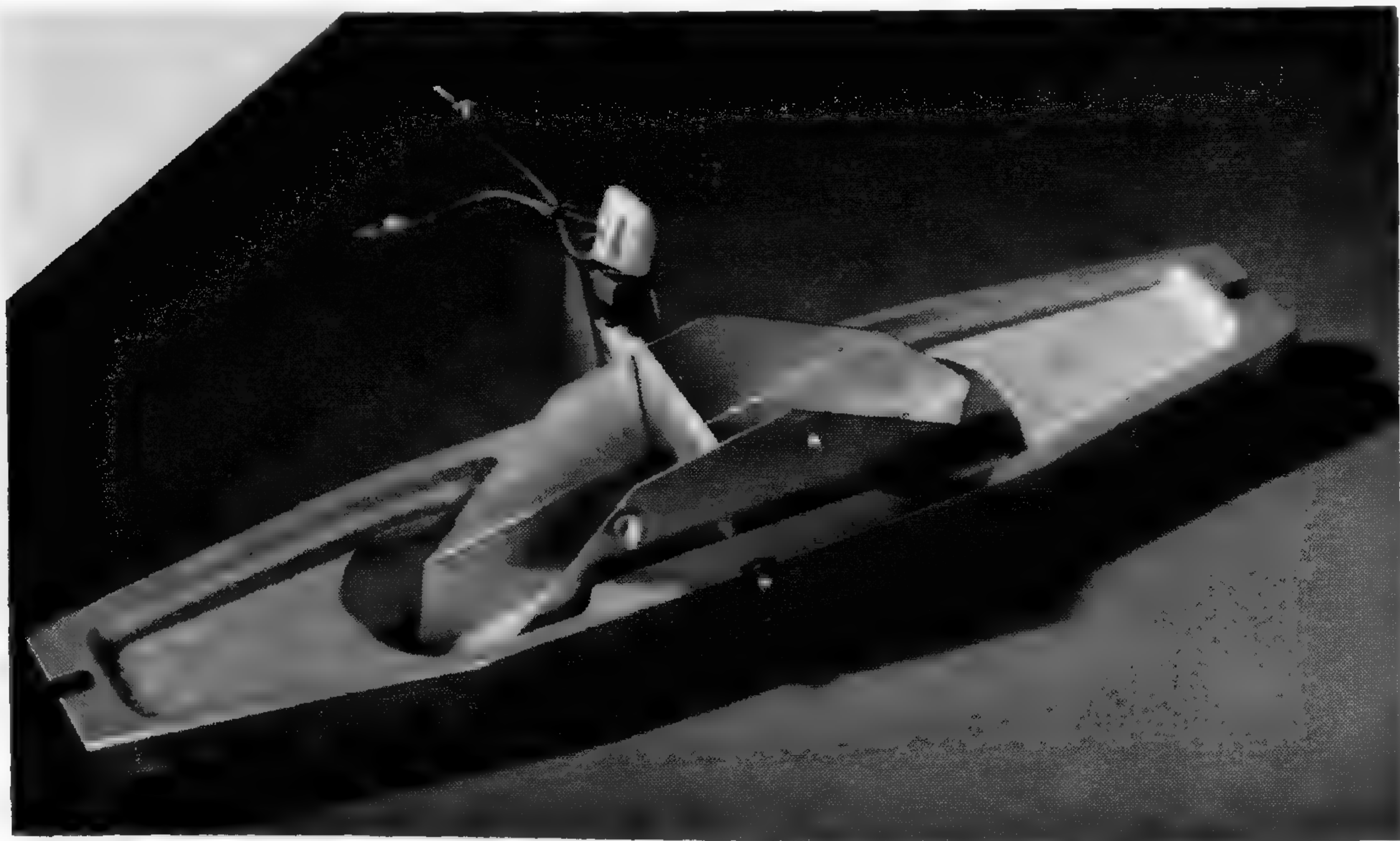
FIG. 6. Tipping bucket mechanism housed inside rain-gage directly under funnel from collector. When one compartment fills bucket tips, closing switch and simultaneously positioning other compartment under funnel.
