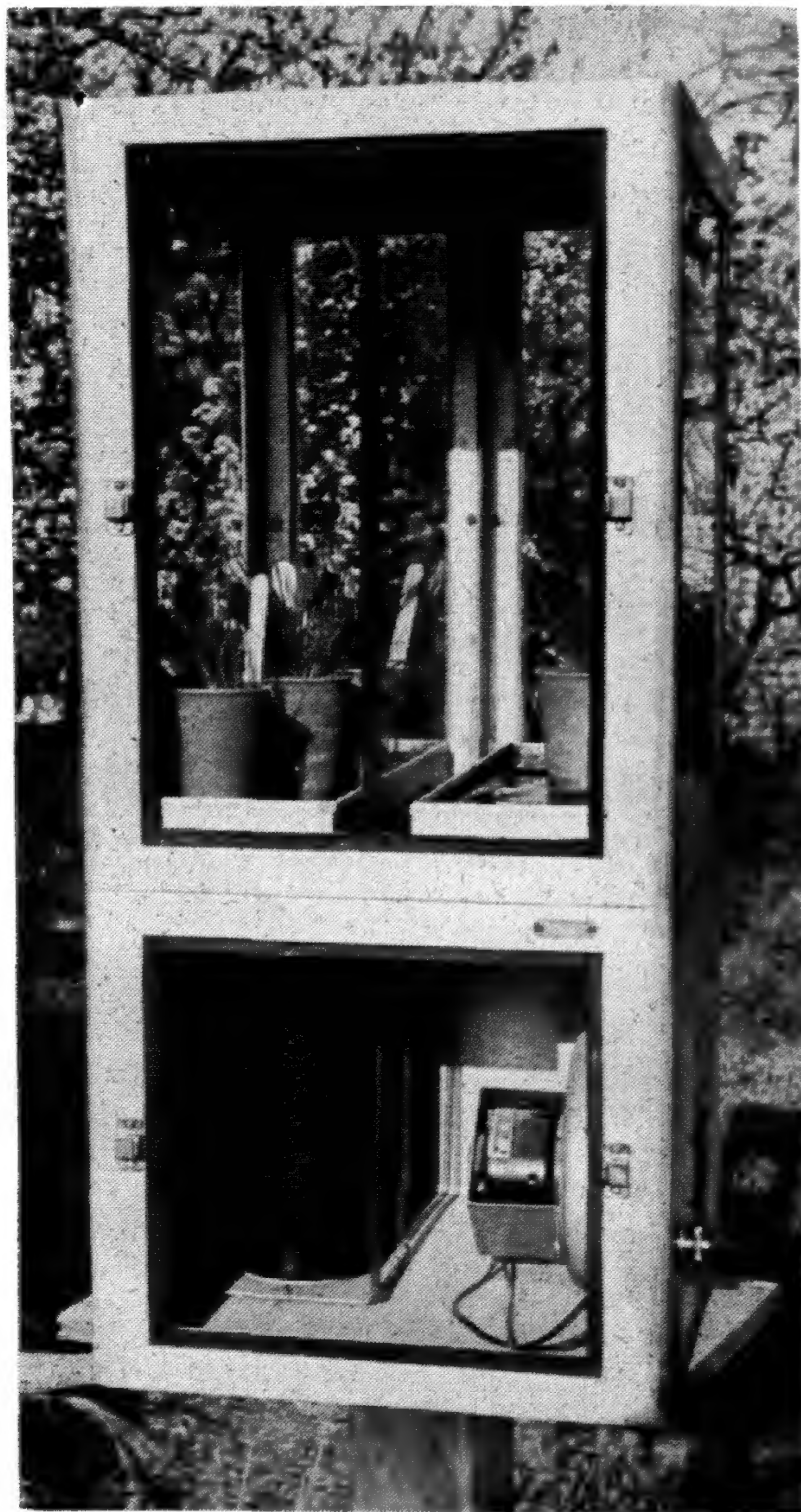
Fig. 1. A test cabinet with covers removed to show: Top, left, filtered air compartment and top, right, unfiltered air. Bottom, right, carbon canister and left, electric blower
