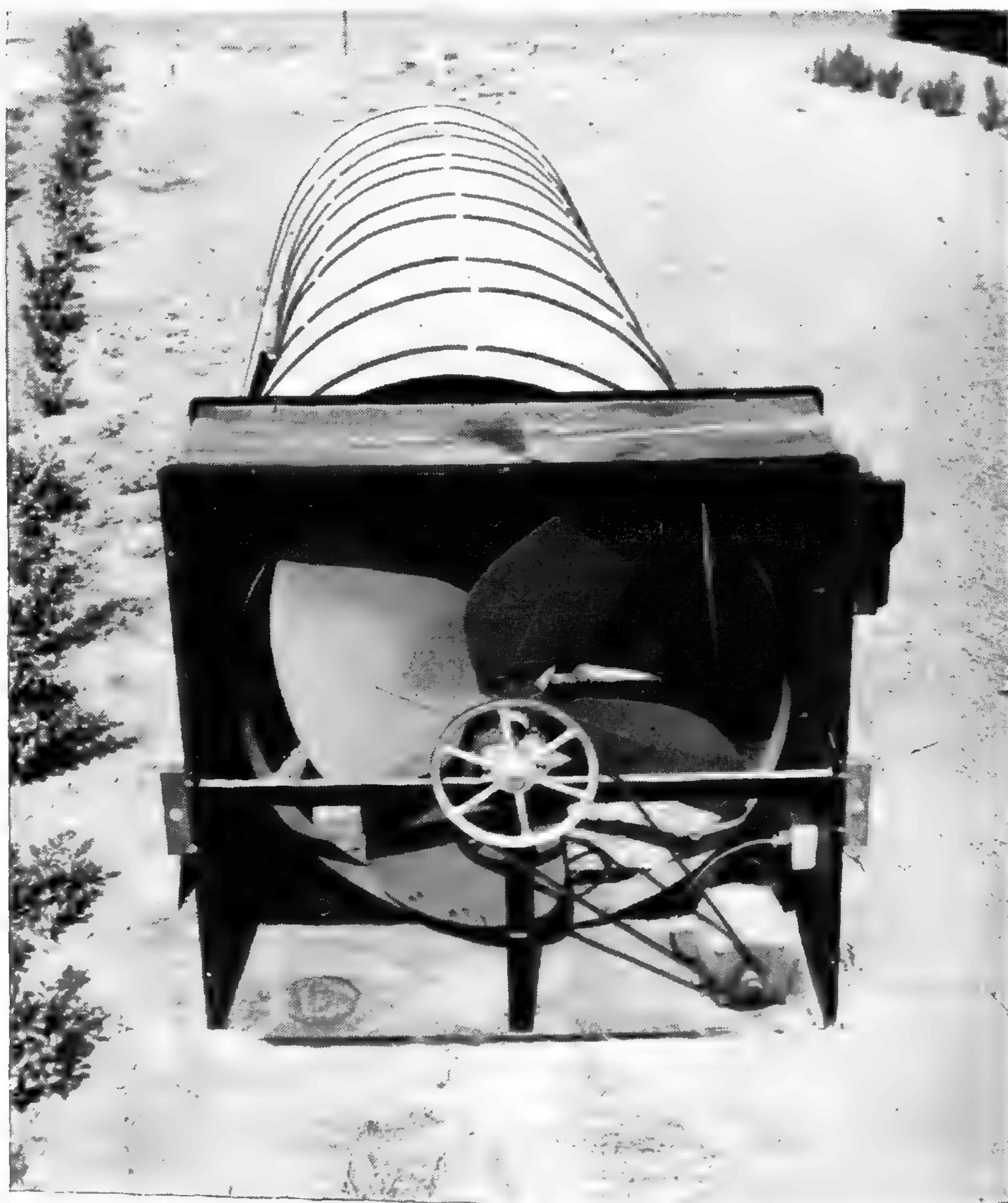
Figure 2. Fire tunnel with 50" electric fan in operational position. Portable generator and propane gas burner not shown.
