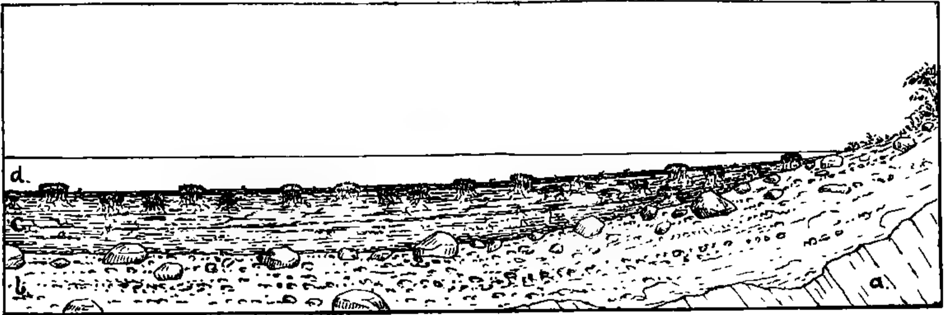
FIG. 30. Theoretical section of bed of lake. a , gneiss; b , gravel and boulders; c , mud and silt; d , water.
