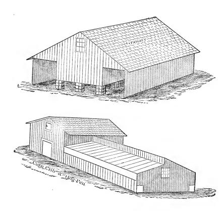
The roof on south side of hog pen drops fifteen inches lower than north side. Boards are hung on hinges so they can be raised to let the sun into the north pens over the south roof, and under eaves of south roof to let sun in south pens.
