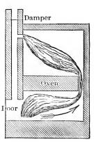
When the fire is being kindled the damper is kept open, the fuel put in by handsful and allowed to burn to a coal. When it ceases blazing the door and damper is closed, and the heated air retained in the furnace. The furnace herein illustrated cost twenty-five dollars. Suitable castings are kept by many of our leading stove dealers. When not, they may be ordered from the manufacturers. The dimensions of this furnace are five and one-half feet long, seven feet high. and twenty-eight inches wide.
