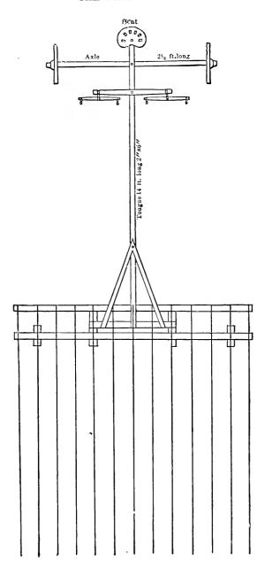
strike the uprights, the hay falls off on the stack. The weight, W, must be a little lighter than the rake, so that the rake in descending, will draw it up. This weight assists the horse to start the load, and continues to assist him, until it strikes the ground. As the load is drawn up from this point, the weight is again raised, and is thus suspended in the air ready to draw the rake down as soon as the horse is backed up.
