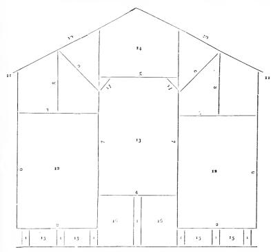
One section of frame, with no sills to catch water and rot out. Each section is set on seven large cedar posts (1), two feet below the surface, and two feet above. Center post five feet above surface.
