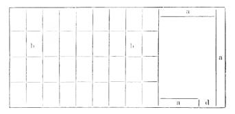
a a a—Boxes for nests. d—Door. b b—Rack for roosts, with slats 3 inches wide, 18 inches apart. Three windows in front of roost, 3 feet long, 8x10 sash, 3 feet from floor. Two feet above this window, a second window, 10x14 sash.
