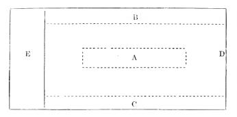
A—Hay rack in center, 4 feet. B—Side hay rack, 3 feet wide. C—Grain trough. D—Double Doors. E—Granary, shingle roof.
