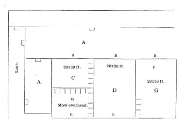
The above is my plan of a barn, sixty by thirty, and sixteen feet posts. A, is barn yard; B, doors; C and G, stabling, which can be made with the mangers as desired; D, threshing floor; F, grain bins; E, mows over head.
