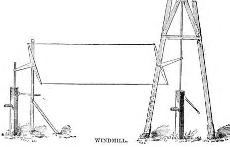
I pump water for the cattle from a well that is sunk several rods from the mill. I use fence wire from the windmill to the pump, in the manner designated by the sketch. As the pump pole works up and down to the mill, it works a T at the mill attached to wires. There is a similar T at the other pump, and both are worked together.
