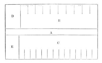
A-Passage for feeding, 4 feet wide. B—Stable for cows, with stanchions. C—Stable for feed cattle, with stanchions, 3 feet wide. D—Box stall for cow at calving time. E—Corn crib, 6x10 feet.
