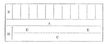
A—Passage for feeding, 3 feet wide. B.—Pens for brood sows, 6½x10, with window in each 3x4, 3 feet from the ground. C—Floor 11 feet wide for feeding on. D—Corn crib, 7x11 feet. E E—Water trough, on main floor.
