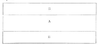
A—Drive way, 9 feet 6 inches wide on floor, 8 feet at top of cribs; difference in width of drive way at top and bottom, to give better circulation of air. B B—Cribs, 7 feet 3 inches at bottom, 8 feet at the top. Shingle roof, with ventilator 4x6 feet on top. Double doors closing drive way, hung on rollers. Double matched floor of inch pine.
