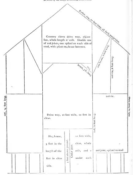
Cribs 2 feet above of ground, no sills; outside underpinning set in one foot.
