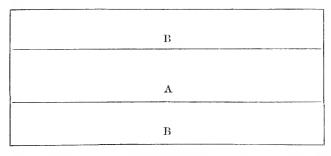
A—Drive way and wagon shed, 10 feet wide. B B—Cribs, 8 feet wide. A tight floor over drive way, forming store room for light farm implements, seed corn, etc. Shingle roof.
