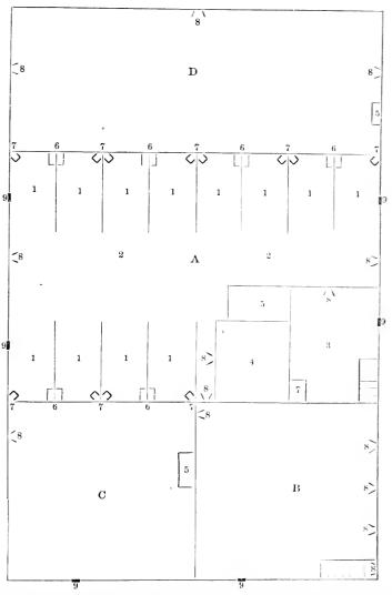
A—Horse part of main barn,  $30\times40$  feet. B—Wagon and carriage stalls,  $20\times30$  feet. C—Calf and sheep shed,  $20\times30$  feet, D—Shed,  $20\times40$  feet. 1—Single stalls,  $5\times10$  feet. 2—Floor between stalls,  $10\times40$  feet. 3—Room for meal and cutter,  $10\times10$  feet. 4—Harness room,  $6\times7$  feet. 5—Water troughs. 6—Hay chutes, extending to upper story. 7—Feed boxes. 8—Doors. 9—Windows.
