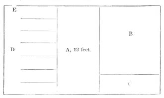
A—Drive way, 12 feet. B—Hay bay, 16x28. C—Corn crib, 6x16. D—Stable, 14 feet wide. E—Entrance, 3 feet wide. Shingle roof, with ventilator on top, 6x8 feet.
