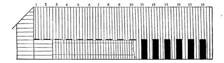
My hog house is ninety-six feet long, and six feet wide. It is boarded up and down with twelve foot lumber, which is sawed in two, so as to give the roof the proper slope; that is, the shorter side about five and one-half feet high, the longer, six
