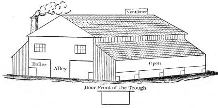
The tank is connected by a pipe to a windmill pump, so that water can be run into the tank, boiler, or troughs, at will. The troughs run the whole length of the pens, on each side of the alley. The pens are double, and the front part or section is used for feeding, and the rear opens into the yard for the removal of the offal, which is easily cleaned out by throwing it through the small door below the space marked "Open." The door front of the trough is hung by a round tenon at
